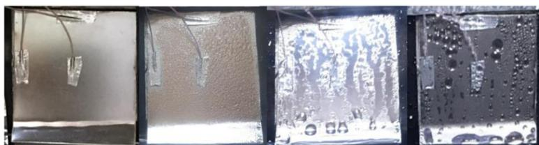
**Figure 4:** Condensation stages from left to right, 1) before steam enters the chamber, 2) initial condensation (fogging and small drop formation), 3) drop coalescing into drips, and 4) condensate load on plate observed at the end of the experiment.
