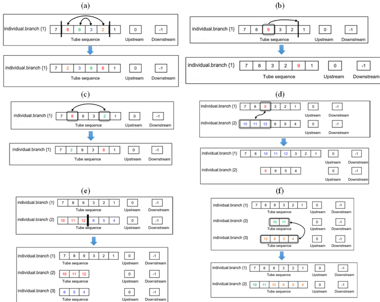
Figure 3: GA Operators: (a) Gene sequence inversion; (b) Gene insertion; (c) In-branch transposition; (d) Cross-branch transposition; (e) Branch detachment; (f) Branch union.
