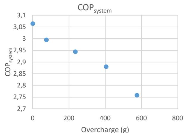
**Figure 6:** Evolution of the system COP in function of the charge
