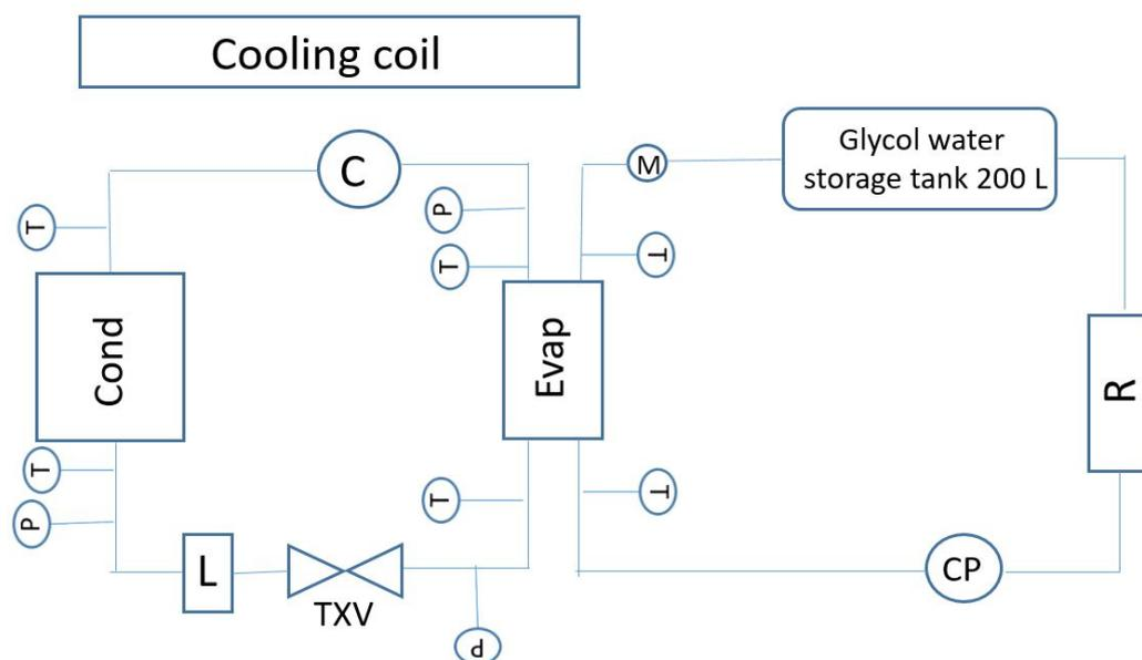
**Figure 1:** Experimental setup for the climatic room, the water-glycol loop and condensing unit.
