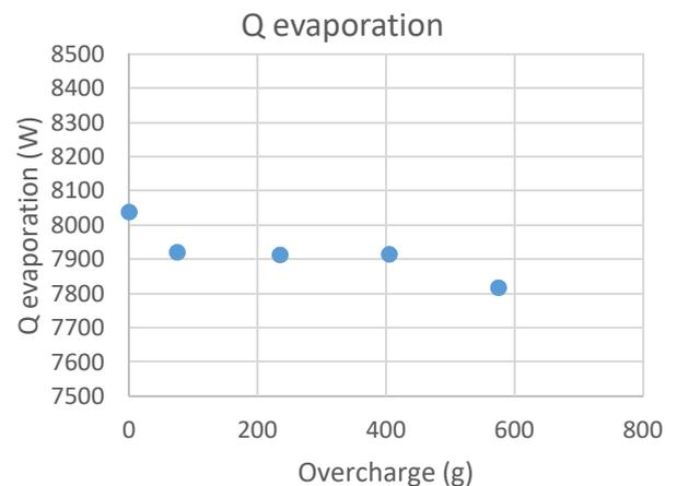
**Figure 4:** Evolution of the cooling capacity in function of the charge
