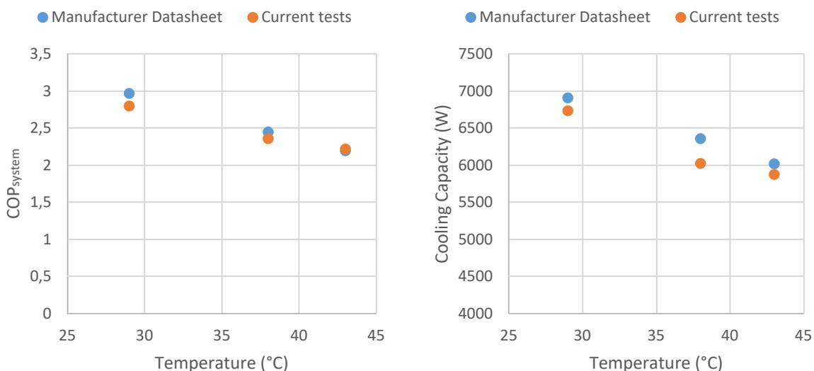
**Figure 2:**  $COP_{system}$  and cooling capacity (W) comparison of current tests with R-134a with manufacturer datasheet at  $T_{evap} = -2.5^\circ\text{C}$  (before overcharging)
