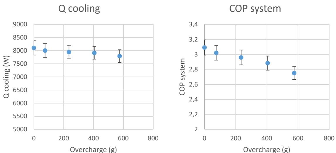
**Figure 7:** Cooling capacity and COP system with error bars
