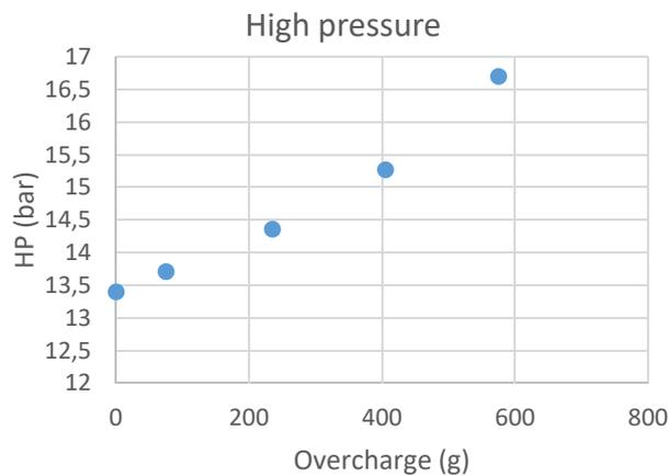
**Figure 3:** Evolution of the high pressure in function of the charge
