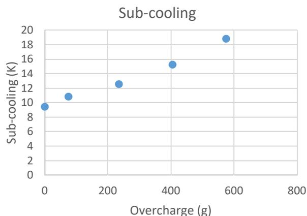
**Figure 5:** Evolution of the sub-cooling in function of the charge
