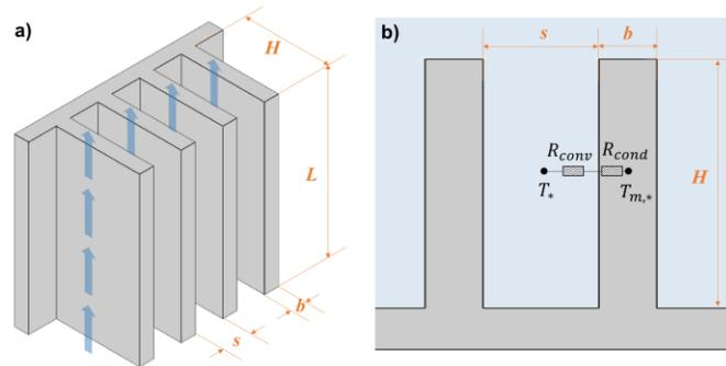
**Figure 2:** (a) Geometric parameters of finned surface design and (b) heat transfer model for the LHTES units.
