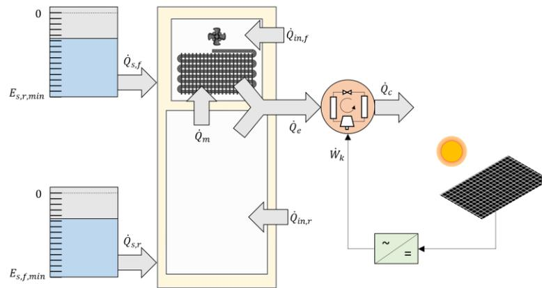
**Figure 1:** Schematic illustration of energy interactions during charge for a household refrigerator driven by photovoltaic power and with latent heat thermal energy storage.
