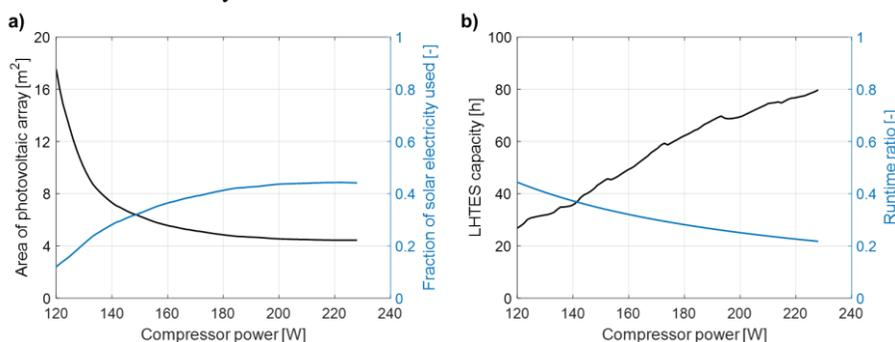
**Figure 3:** (a) photovoltaic array size and energy utilization, and (b) LHTES capacity and compressor runtime ratio.
