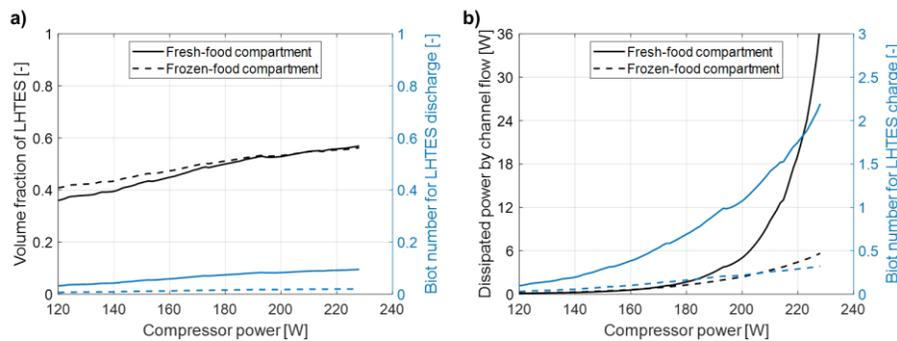
**Figure 4:** Design parameters for LHTES units associated to (a) the discharge process and (b) the charge process.
