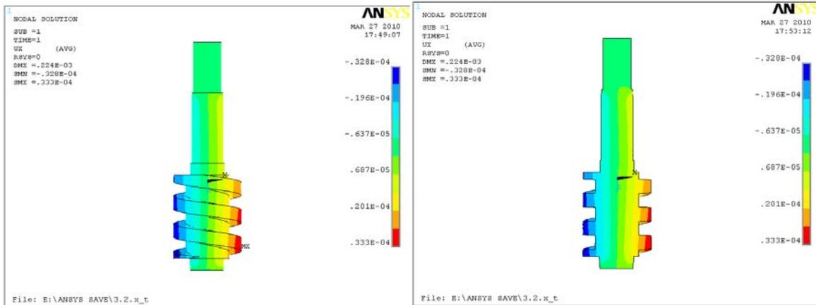
Fig. 4: The deformation of screw rotor in the x direction
