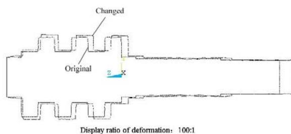
**Fig. 11:** Rotor axial cross section change with GVF 99%
