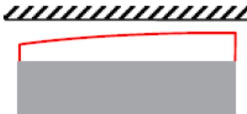
**Fig. 13:**Circumferential gap changes (the shaded shows change before, red line shows changes)
