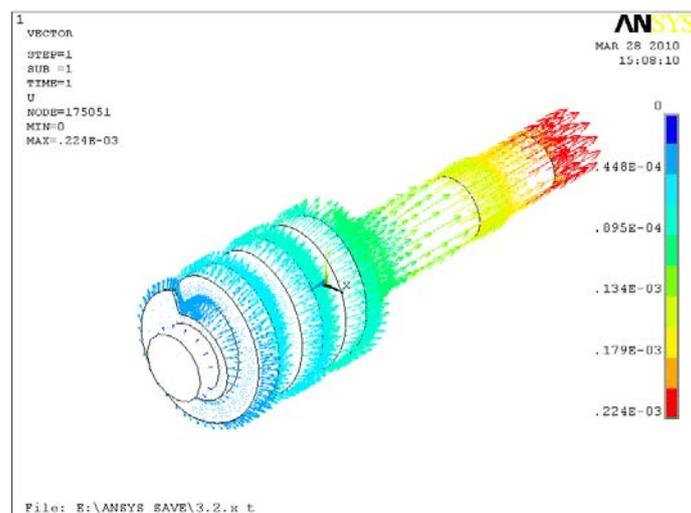
**Fig. 7:** Vector representation of screw rotor deformation
