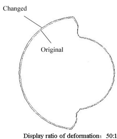
**Fig. 8:** Rotor profiles change with GVF 80%
