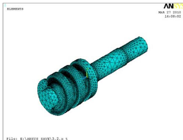
**Fig. 2:**The finite element grid of screw rotor
