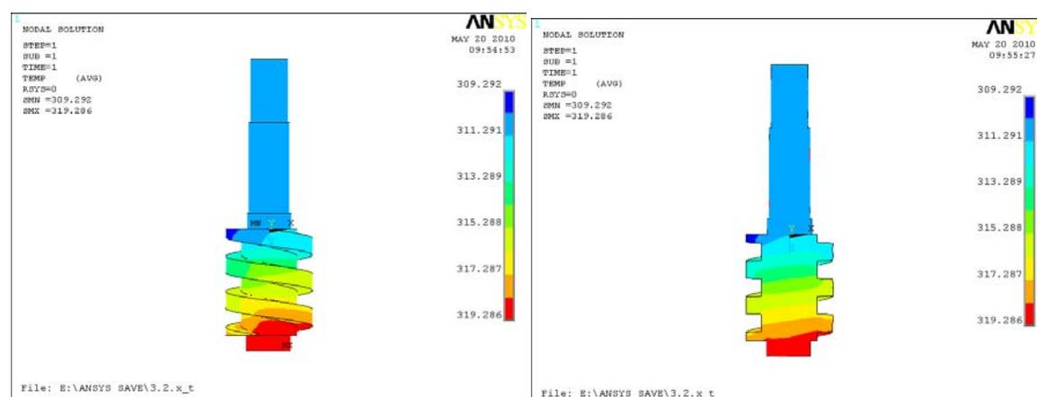
**Fig. 3:**Temperature distributions of the screw rotor
