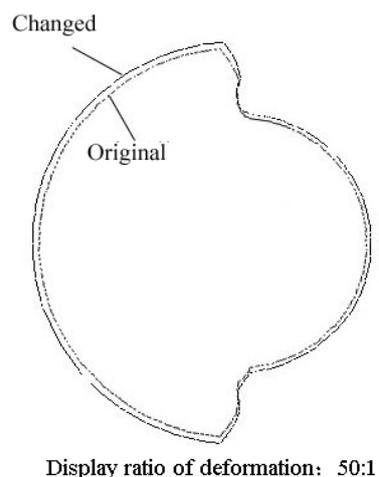
**Fig. 9:** Rotor profiles change with GVF 99%
