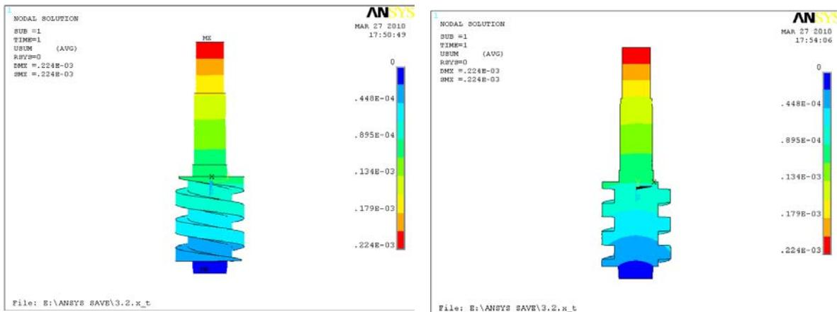
Fig. 6: The comprehensive deformation of screw rotor
