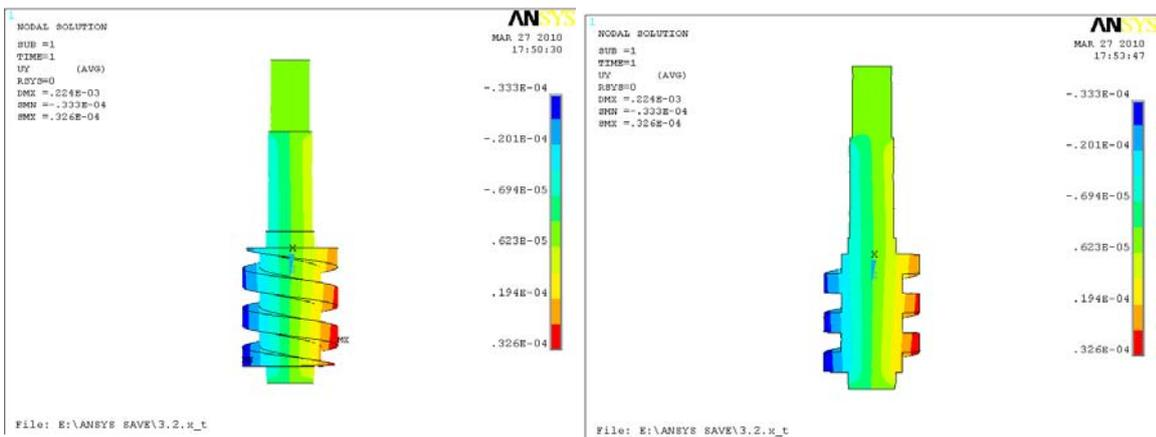
Fig. 5: The deformation of screw rotor in the y direction
