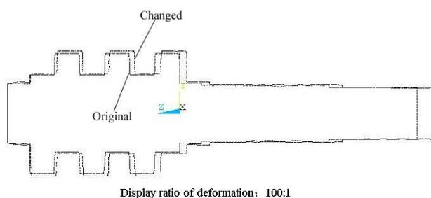
**Fig. 10:** Rotor axial cross section change with GVF 80%
