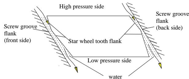
**Figure 3:** Schematic diagram of the meshing pair
