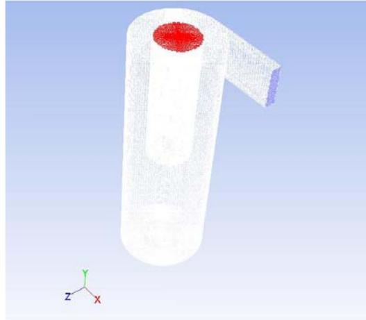
Fig.3 The computational grid for the cyclone separator
