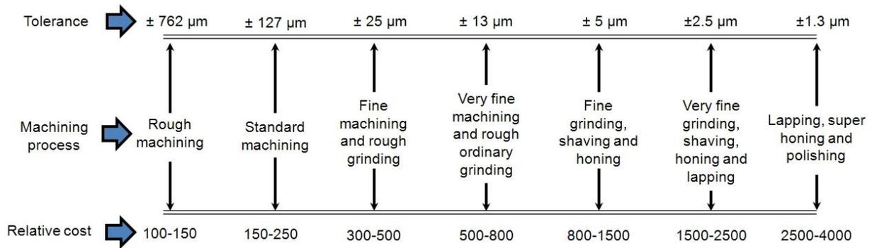
**Figure 3:** Relative cost x machining process x tolerance (from Rao, 1992)
