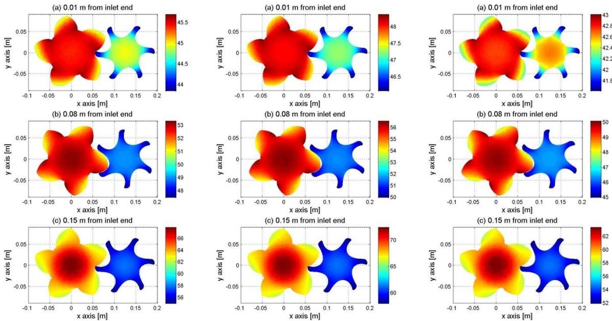
**Figure 7:** The calculated rotor temperature distributions
