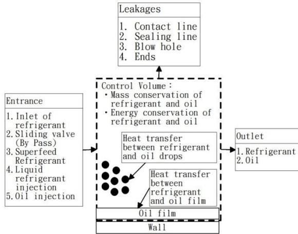
**Figure 2:** The physical model of lumped parameter analysis
