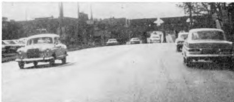
Fig. 7. Shows extra wide curb lane with parking with remaining width not adequate for moving traffic.
