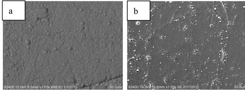
Figure 1. Surface appearance (a)Ni-P; (b)DLC
