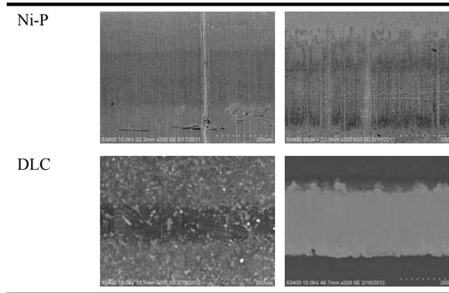
Figure 6. Comparison of grinding crack
