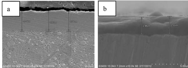
Figure 3. Profile appearance (a)Ni-P; (b)DLC
