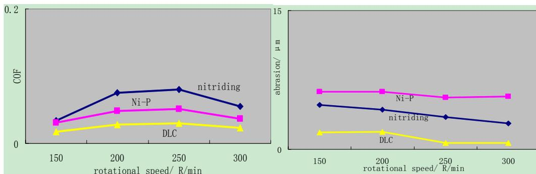
Figure 7. COF and abrasion VS time (200 N, 1 h)
