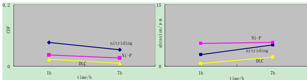
Figure 5. COF and abrasion VS time (200N, 300RPM)
