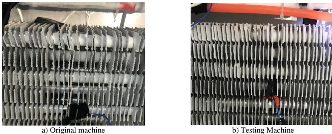
**Figure 2:** Frost on the surface of the evaporator
