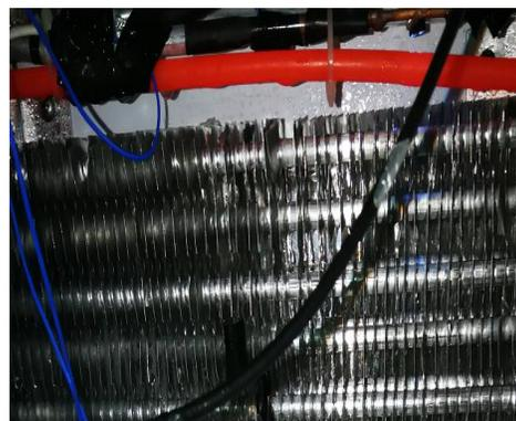
b) Defrosting effect diagram of testing machine
