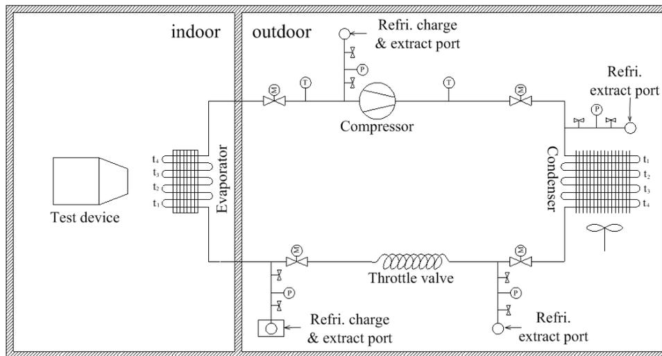
**Figure 1:** Refrigerant distributing test layout
