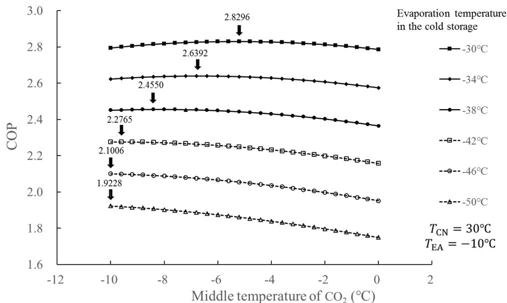
Figure 4: COP versus middle temperature of CO<sub>2</sub> at different evaporation temperature of cold storage
