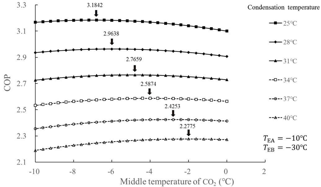
**Figure 2:** COP versus middle temperature of CO<sub>2</sub> at different condensation temperature
