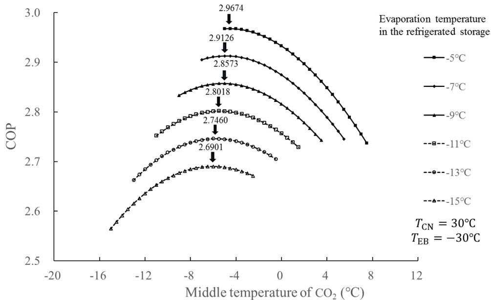
**Figure 3:** COP versus middle temperature of CO<sub>2</sub> at different evaporation temperature of refrigerated storage
