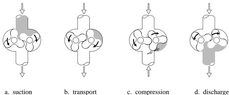
**Figure 3:** Compression cycle of a conventional Roots blower
