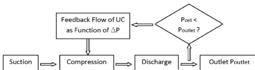
**Figure 8:** Negative feedback loop of UC
