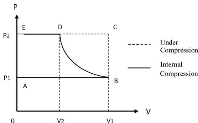
**Figure 2:** UC of Roots blower vs internal compression on P-V Diagram
