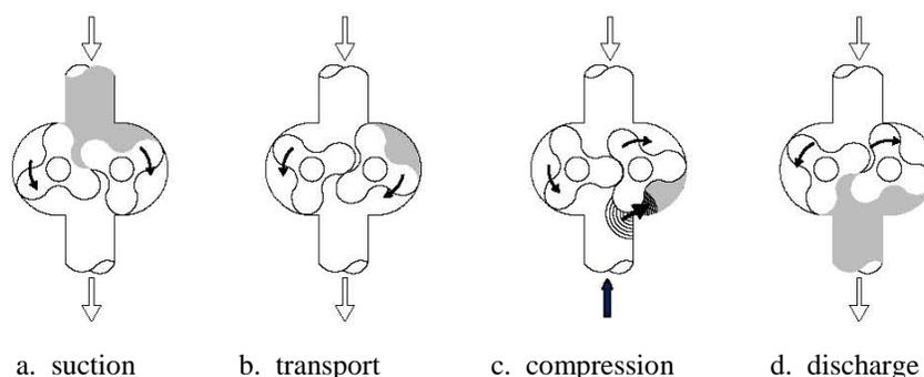
**Figure 6:** Compression cycle of a conceptual Roots blower according to the shock tube theory
