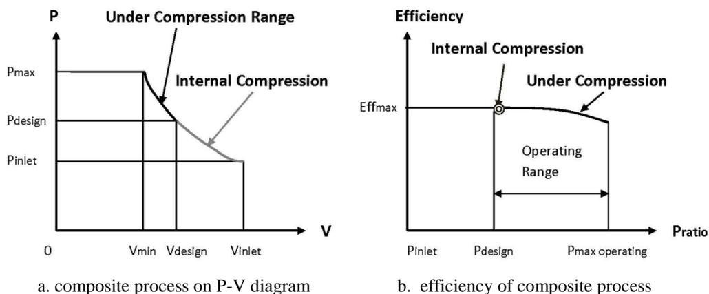
**Figure 9:** Composite process by combining internal compression with UC
