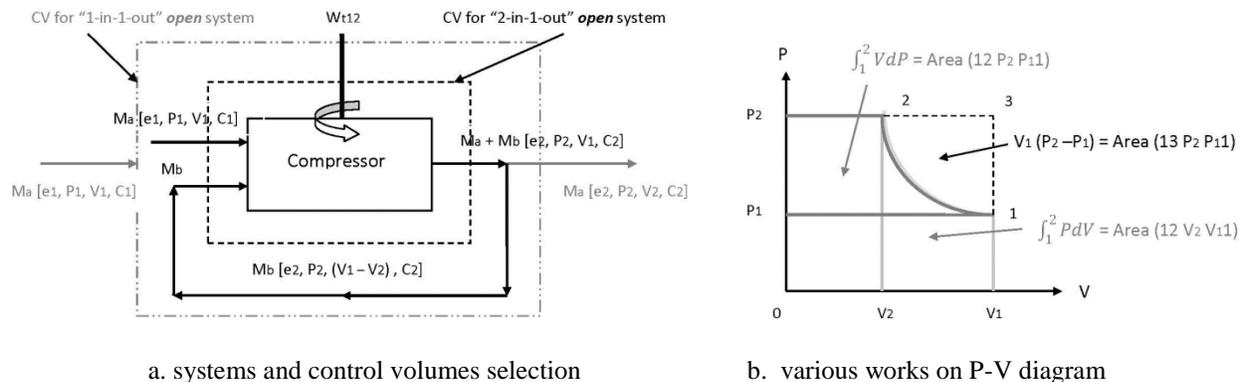
**Figure 4:** Selection of control volumes and works of under compression
