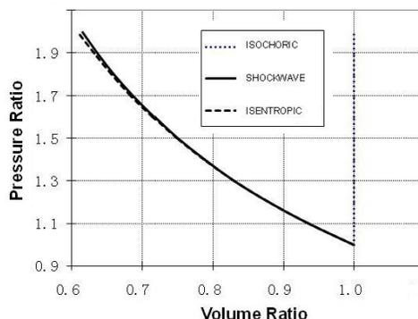
**Figure 7:** Thermodynamic processes of isentropic, shockwave and isochoric processes on P-V diagram
