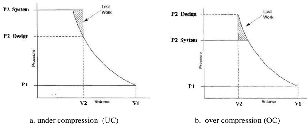
**Figure 1:** UC or OC of PD compressors on P-V diagram
