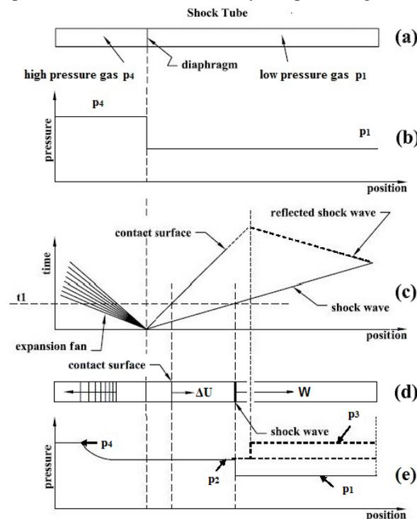
**Figure 5(a-e):** Diaphragm-triggered shock tube wave diagram and pressure distribution
