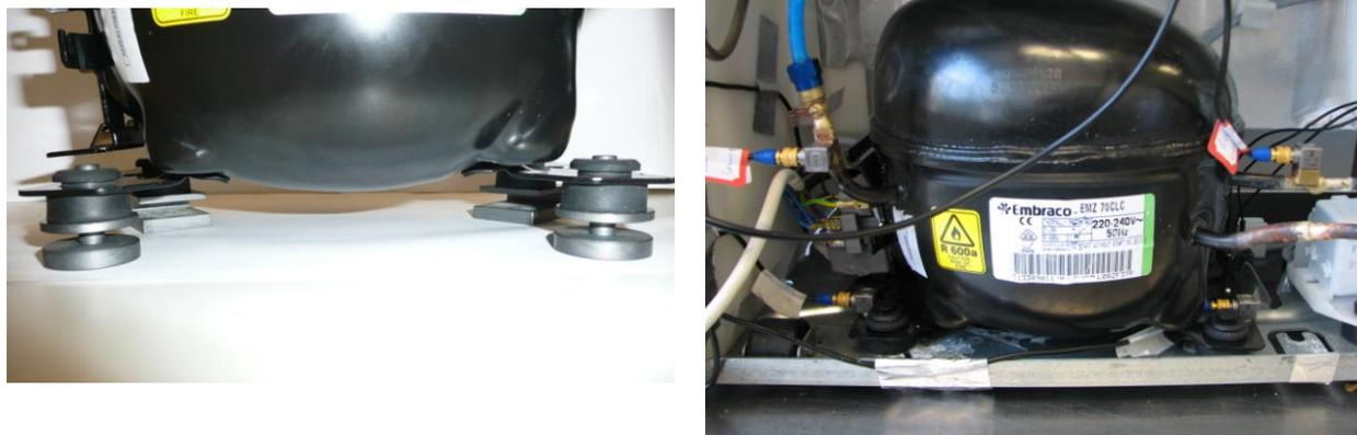
**Figure 2:** (a) Compressor supported on the floor. (b) Flexible tube (plastic) in the suction of the compressor.
