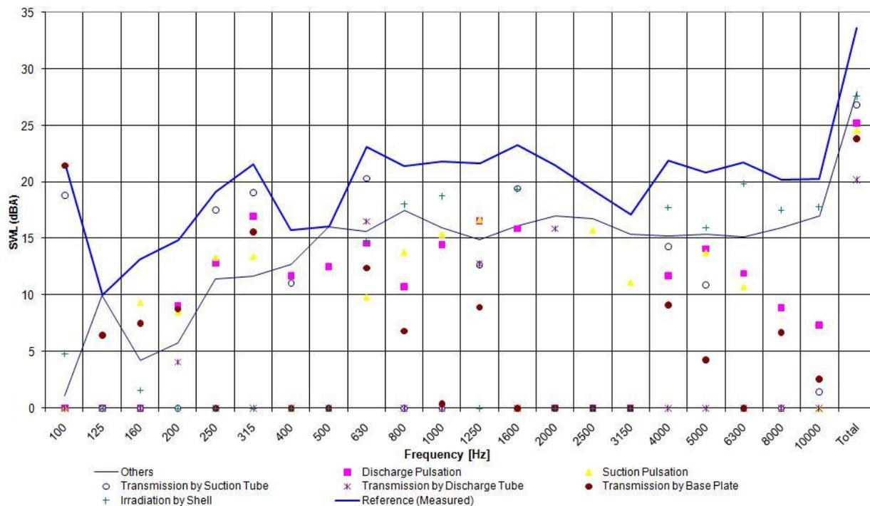
**Figure 4:** Contribution of each energy path in the noise in 1/3 octave band
