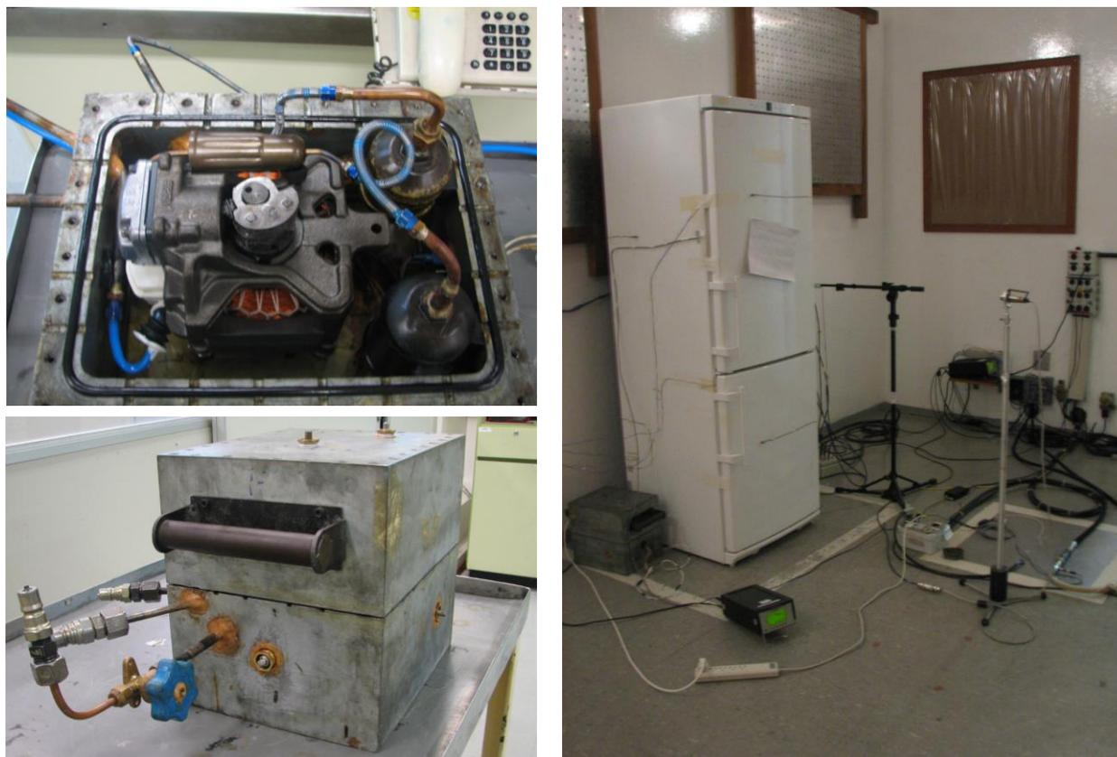
**Figure 3:** (a) Compressor within the steel box. (b) Assembly of the steel box in the system
