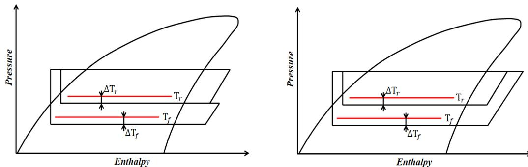
In the two-stage compression dual-evaporator (TSCDE) cycle shown in Figure 1a, low pressure cylinder (LCYL) and high pressure cylinder (HCYL) are piled together and working for different compression missions. Meanwhile
