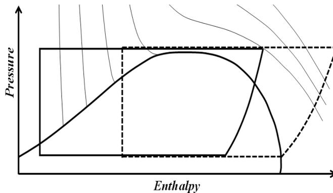
Figure 9: p-h diagrams for HP and PHWC-HP cycles
