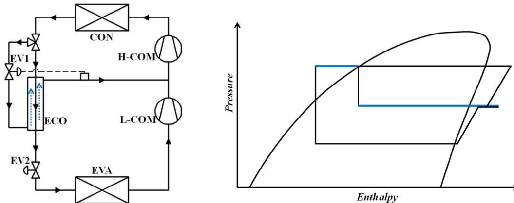
**Figure 6:** Schematic and p-h diagram for SHVIHP cycle
