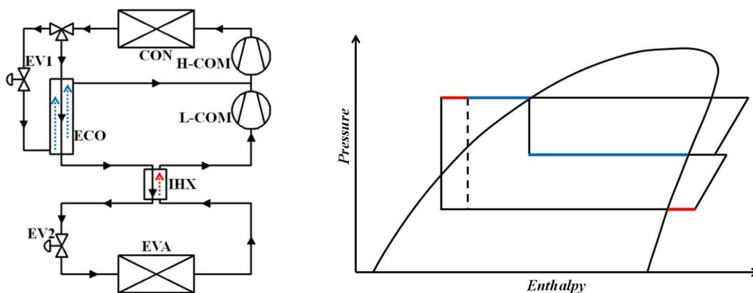
**Figure 5:** Schematic and p-h diagram for IHE-VIHP cycle
