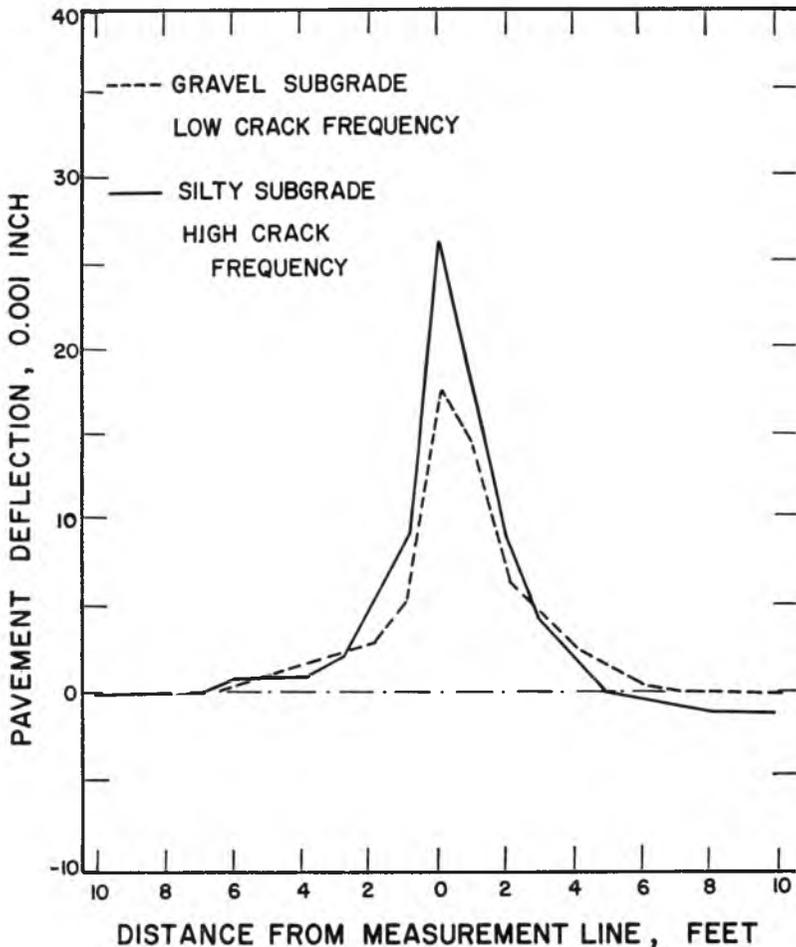
Fig. 4. Typical longitudinal deflection curves.
