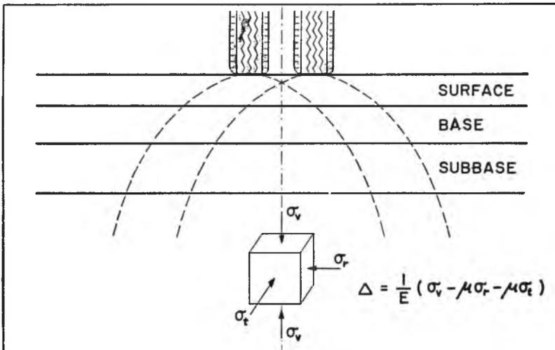
Fig. 5. Idealized stresses and strain under dual wheels.
