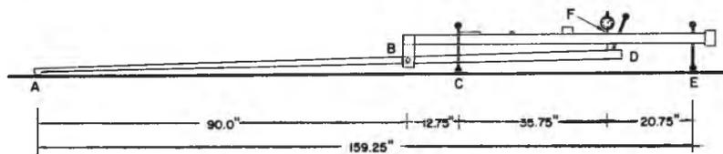
Fig. 7. Diagrammatic sketch of Benkelman Beam.
