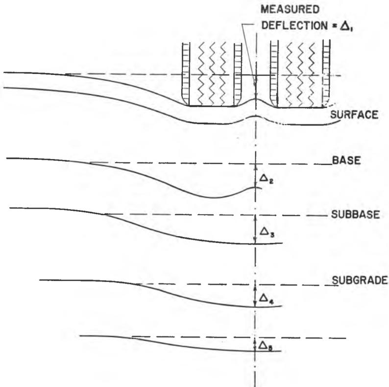
Fig. 1. Deflection profiles under dual wheels.
