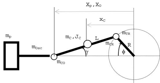
**Figure 4:** Crank gear mechanism
