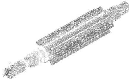
**Figure 6** 3D-Model of rotor shaft of induction motor for 1.4 MW 375 rpm for a four axes horizontal balanced opposite reciprocating compressor B254.
