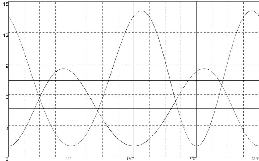
**Figure 3:** Equivalent mass moment of inertia  $J(\phi)$   $\text{kgm}^2$  and average inertia (constant) versus crank angle
