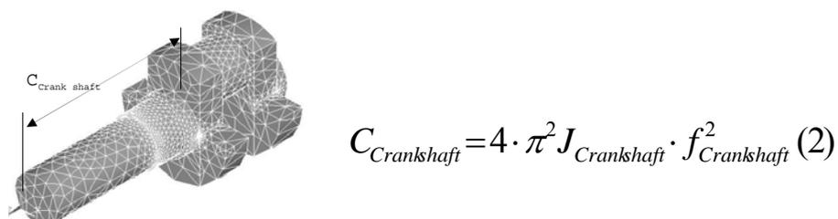
**Figure 2:** Crank shaft torsional stiffness
