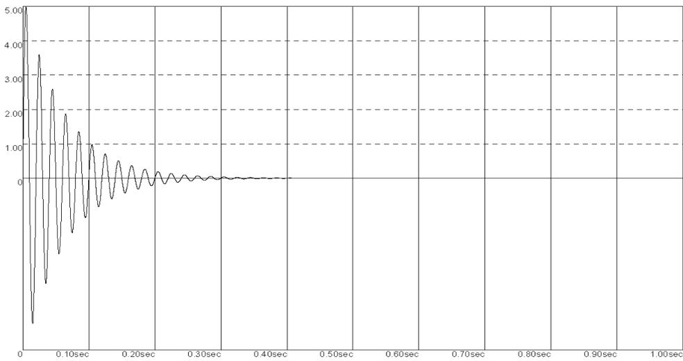
**Figure 8** Ratio of motor short-circuit torque to the rated torque versus time in s.
