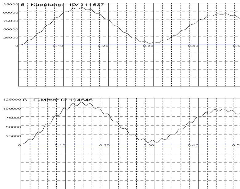
**Figure 12.** Dynamic torque at highly flexible coupling and E-Motor versus starting time in sec.
