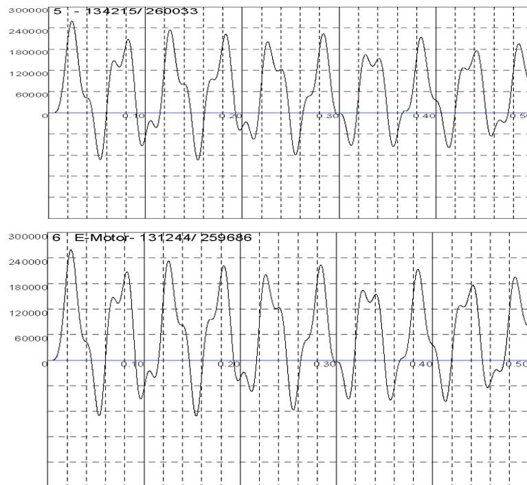
Figure 14. Dynamic torque at stiff coupling and E-Motor versus starting time in sec.
