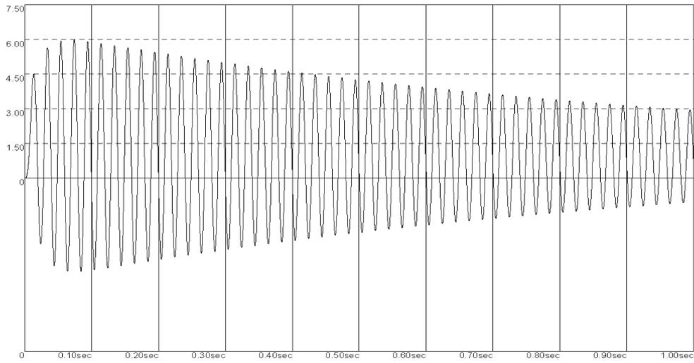
**Figure 7** Ratio between the motor start torque and the rated torque versus time in s.
