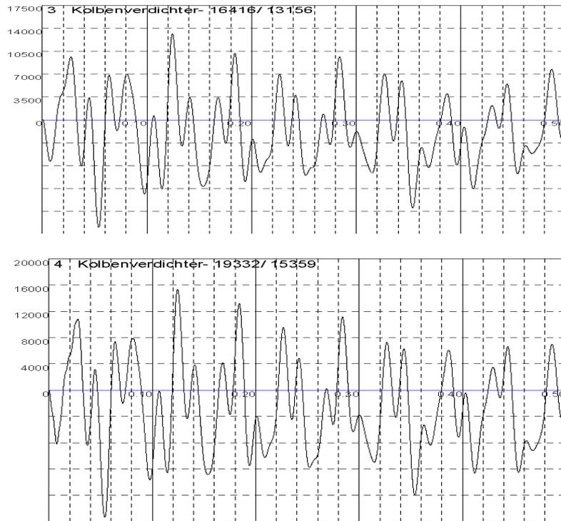
Figure 13. Dynamic torque at crank shaft versus starting time in sec, stiff coupling.
