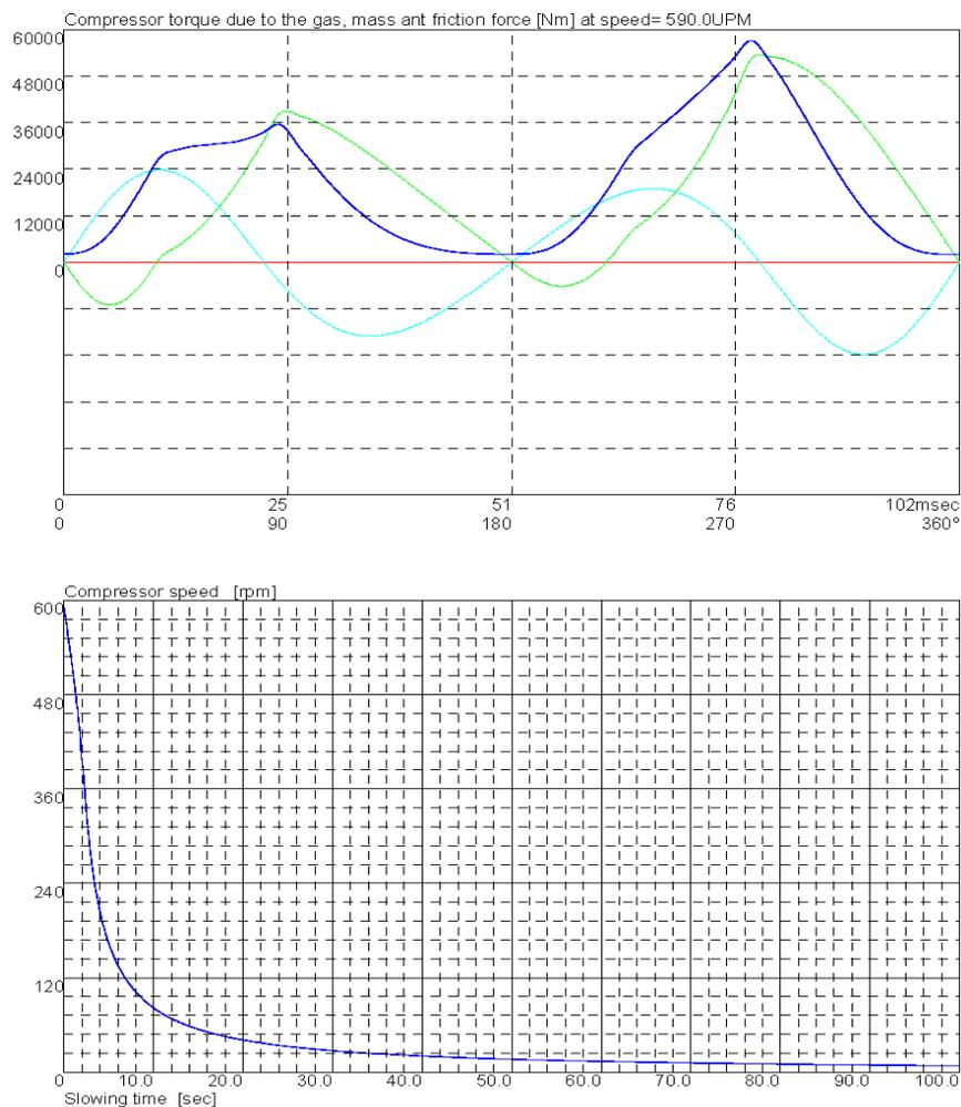
**Figure 15.** Compressor torque at 590rpm and the motor speed over the slowing time.
