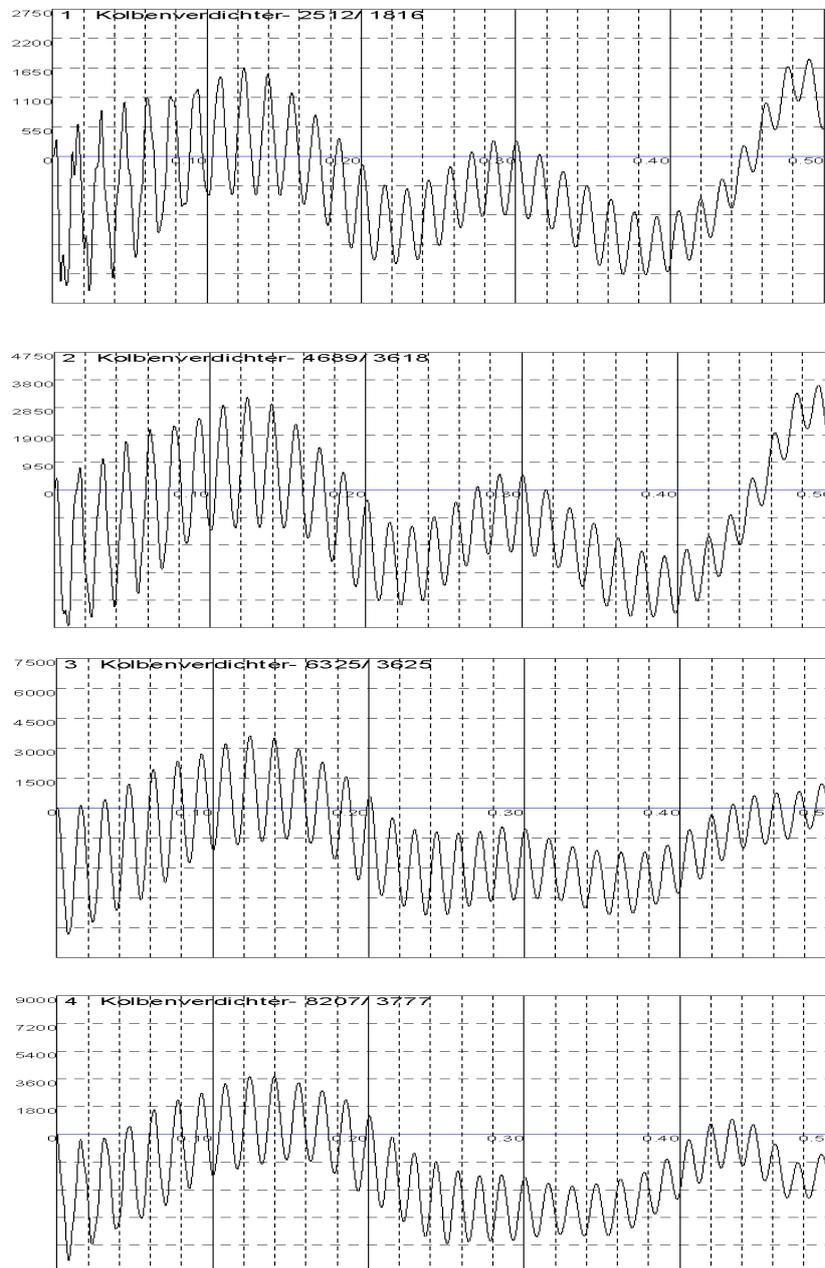
**Figure 11.** Dynamic torque at crank shaft versus starting time in sec, flexible coupling.
