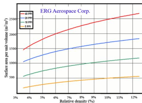
Fig. 2: Surface area per unit volume for different types of metal foams.
