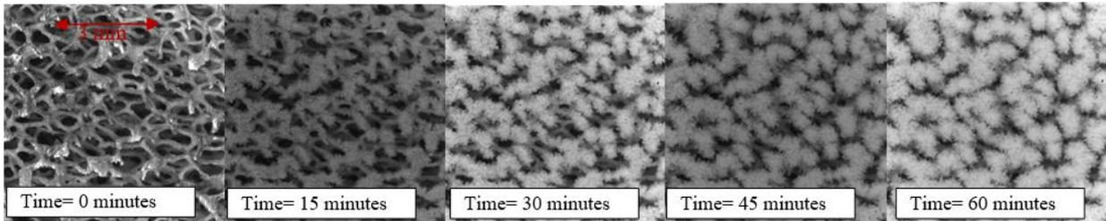
Fig. 13: Frost growth on a 10 PPI copper foam
