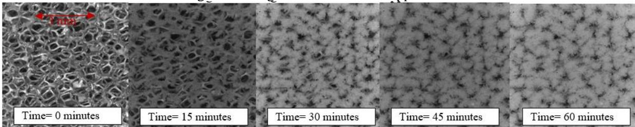
Fig. 14: Frost growth on a 20 PPI copper foam
