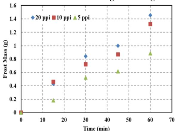
Fig. 16: Frost mass on aluminum foam samples
