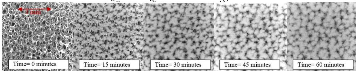
Fig. 15: Frost growth on a 40 PPI copper foam
