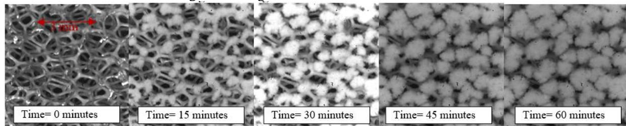
Fig. 11: Frost growth on a 10 PPI aluminum foam
