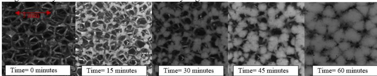
Fig. 10: Frost growth on a 5 PPI aluminum foam
