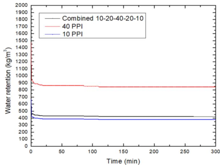
Fig. 8: Water retention for combined samples
