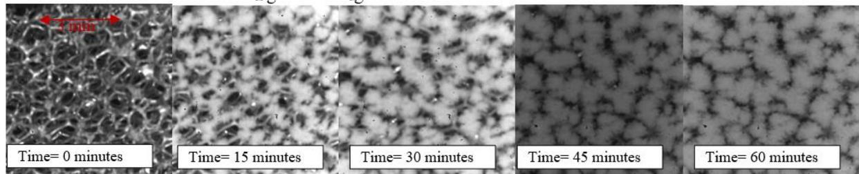
Fig. 12: Frost growth on a 20 PPI aluminum foam
