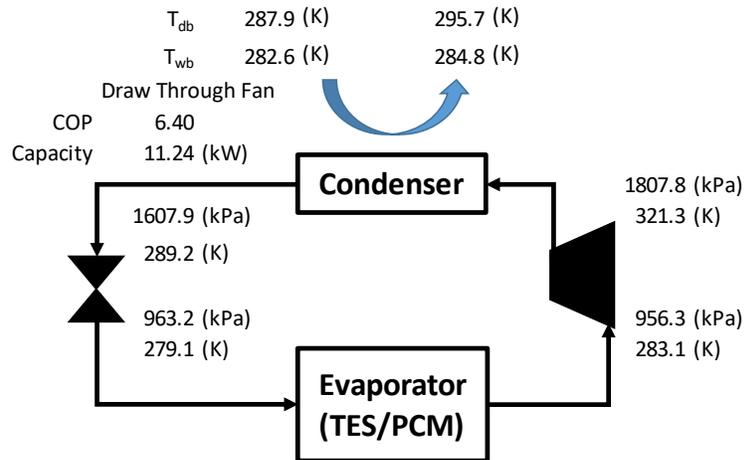
Figure 5. Conditions when TES/PCM charged at 287.9K outdoor temperature
