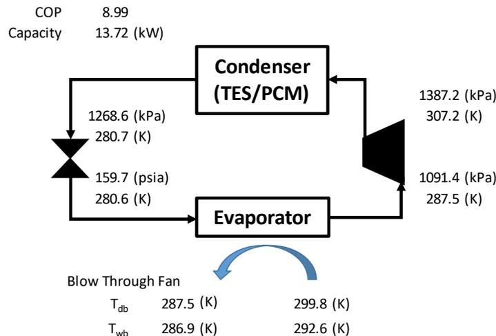
Figure 4. Conditions when system with TES discharged
