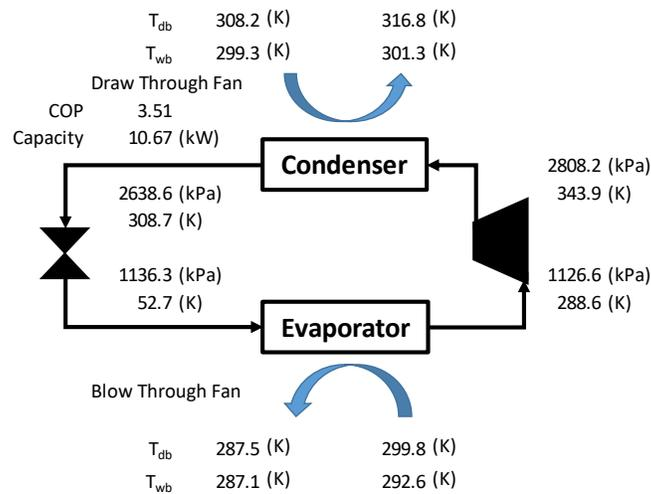
Figure 2. Typical conditions for a R410A residential system as baseline
