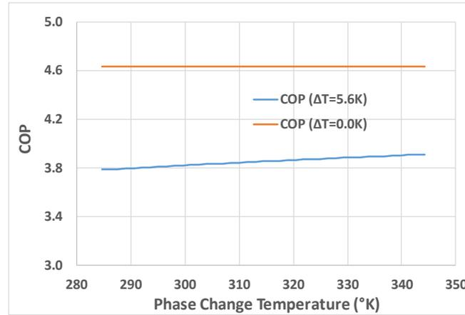
Figure 1. Overall system COP versus phase change temperature for Carnot cycles.  $T_h=344K$  and  $T_c=283K$  are used in the calculation.
