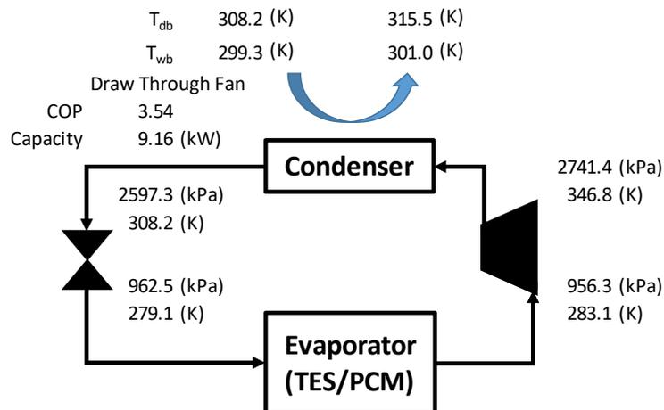
Figure 3. Conditions when TES/PCM charged at 308.2K outdoor temperature
