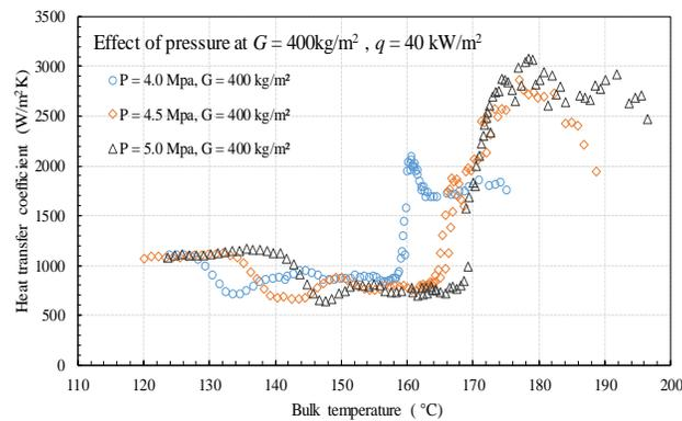
**Figure 2.** Heat transfer deterioration under moderate heat flux
