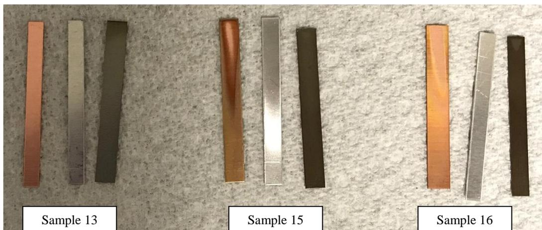
**Figure 10:** Exposed Metal Coupons using HFC-134a
