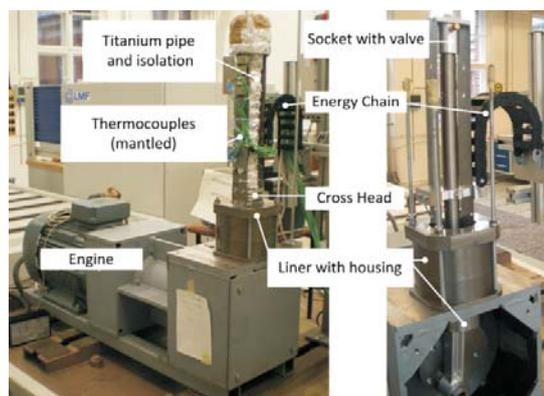
Figure 4: Set up Model Test Rig "Alpha"
