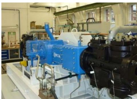
Figure 10: Balanced opposed compressor
