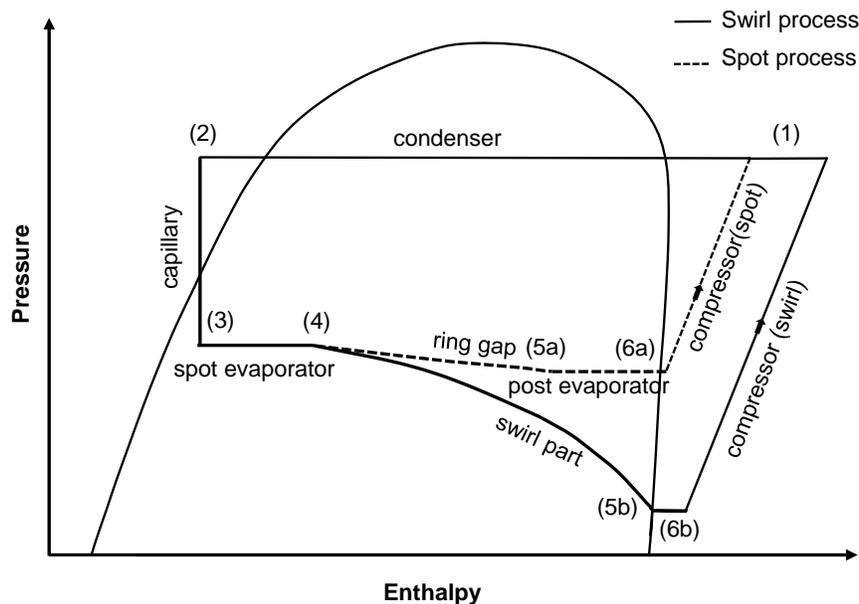
Figure 3: Cycle process diagram
