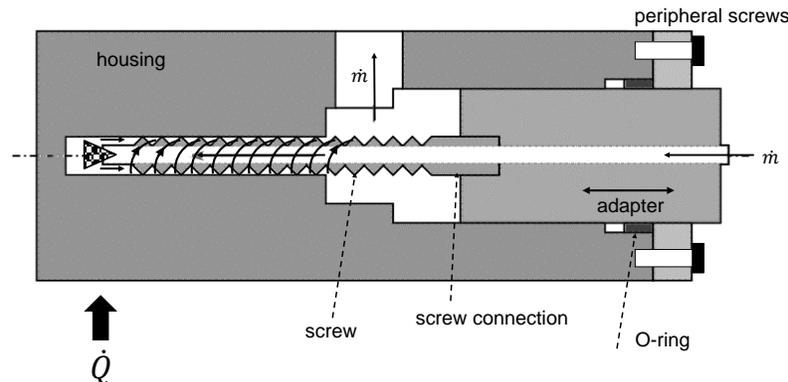
**Figure 9:** Swirl evaporator with variable screw engagement length
