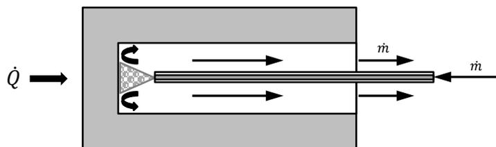
**Figure 1:** Spot evaporator
