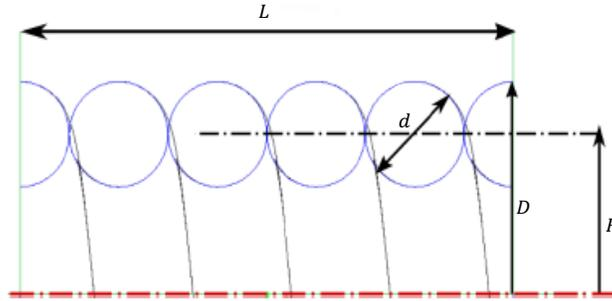
**Figure 4:** Geometric sizes of the swirl insert
