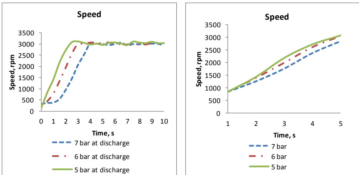
**Figure 7:** Speed curves for start modes with different discharge pressures
