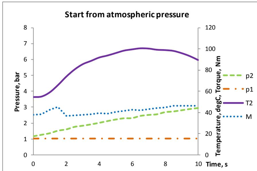
Figure 3: Start from atmospheric pressure at discharge
