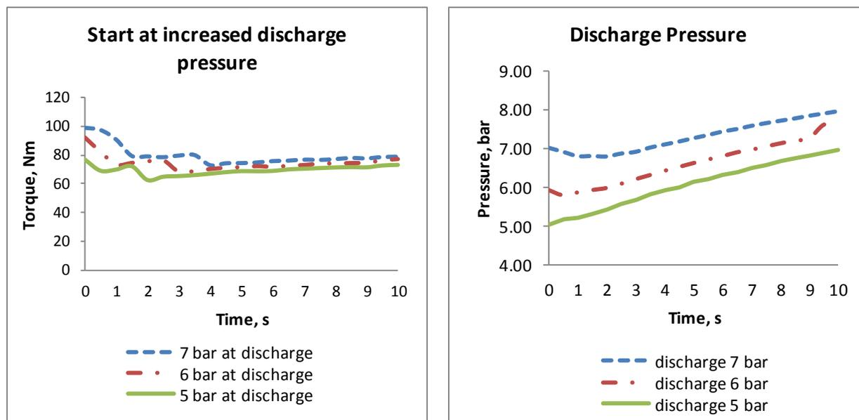
**Figure 8:** Torque and discharge pressure curves for starts with different discharge pressures
