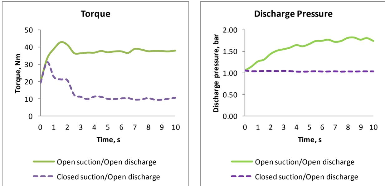
**Figure 6:** Comparison of start with open and closed suction
