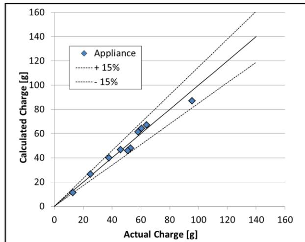
Figure 2: Results of charge estimations using engineering equation
