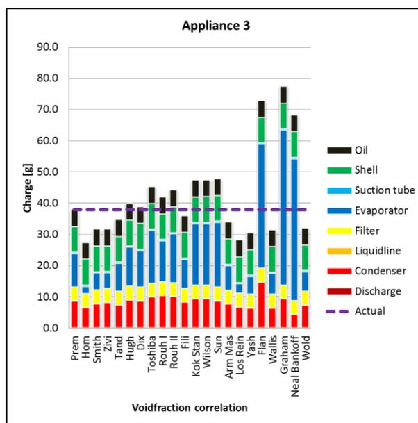
Figure 1: Results of charge estimations for appliance (bottle cooler with storage volume of 500 dm<sup>3</sup>).
