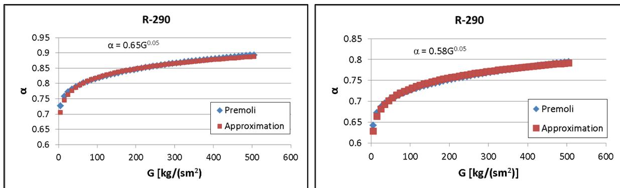
Figure 4: Calculation and approximation using power function of the average void fraction using the slip ratio correlation of Premoli *et al*, 1970, for a tube with inner diameter of 5 mm. Left evaporator. Right condenser.
