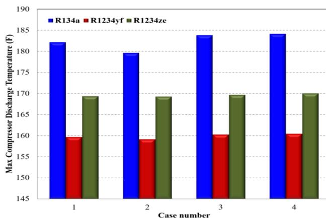
Figure 12. Max compressor discharge temperature for different refrigerants with varying design options
