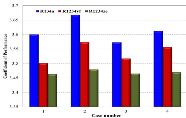
Figure 9. Coefficient of Performance (COP) for different refrigerants with varying design options
