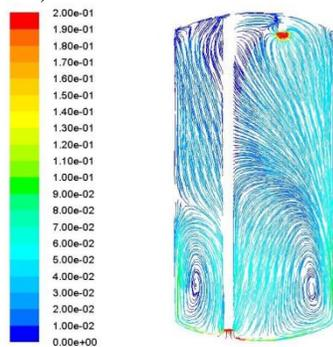
Fig. 2. Streamline for water flow in the tank during draw (scale shows velocity in m/s)
