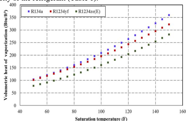
Figure 7. Volumetric heat of vaporization at different saturation temperatures
