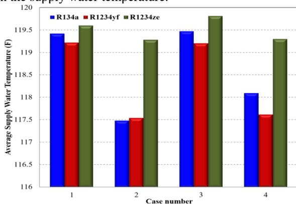
Figure 10. Average supply water temperature for different refrigerants with varying design options
