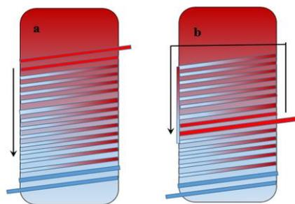
Fig. 4. Condenser wrap configurations: (a) counterflow, (b) parallel-counterflow.
