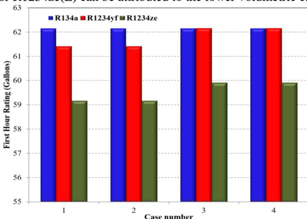
Figure 6. First Hour Rating for different refrigerants with varying design options
