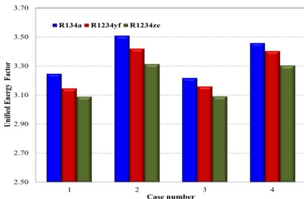
Figure 8. Unified Energy Factor (UEF) for different refrigerants with varying design options
