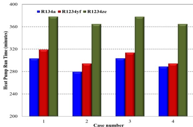
Figure 11. Heat pump run time for different refrigerants with varying design options
