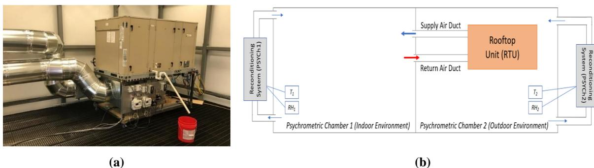
**Figure 2:** (a) Packaged rooftop air conditioning unit installed at Herrick Laboratories (Patil, 2018)
