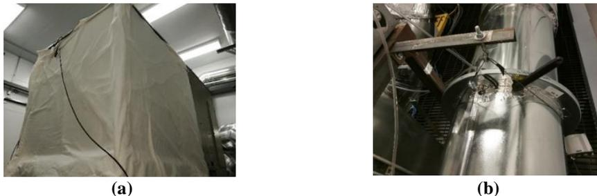
**Figure 3:** (a) Light Condenser fouling simulated by a layer of fabric placed on the condenser surface
