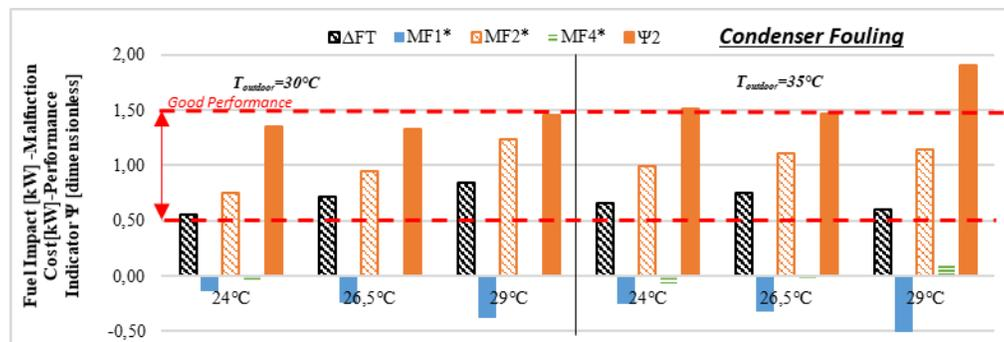
**Figure 4:** Condenser fouling: sensitivity analysis of the technique to the outdoor temperature and to return air temperature.
