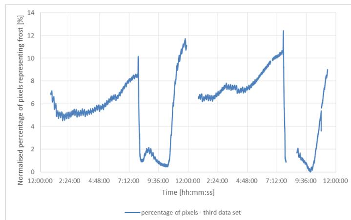
**Figure 5:** Amount of frost on the exchanger surface
