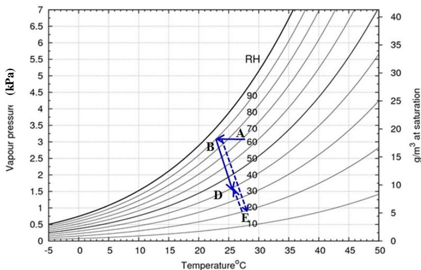
**Figure 2:** Operation of SSLC system (with enthalpy wheel)
