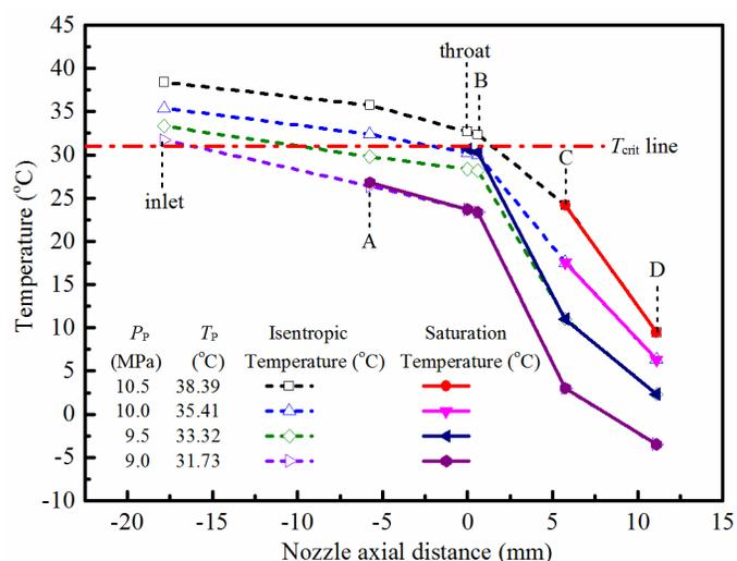
**Figure 7:** Comparison of isentropic temperature and saturation temperature
