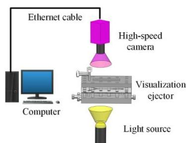
**Figure 3:** Schematic diagram of visualization test platform
