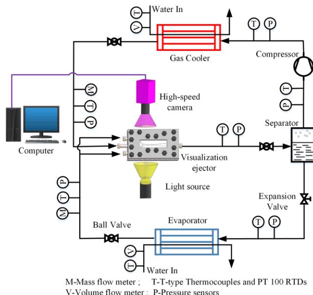
**Figure 1:** Schematic diagram of the transcritical CO<sub>2</sub> EERC
