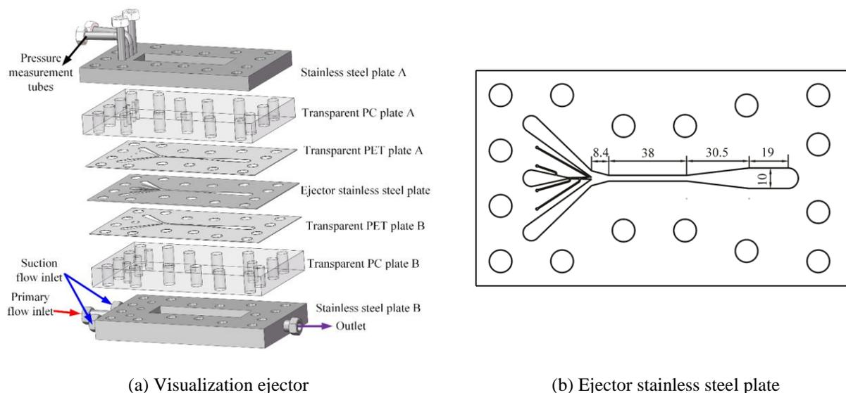
**Figure 2:** Schematic diagram of the visualization ejector
