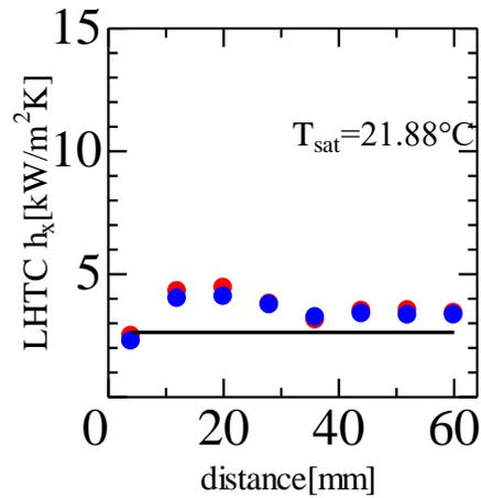
**Figure 4:** Local heat transfer coefficient of condensation (mixture,  $x=0.57$ ,  $G = 10 \text{ kg/m}^2\text{s}$ )
