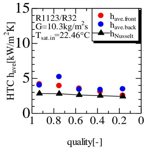
**Figure 6:** Average heat transfer coefficient of cross section (mixture,  $G = 10 \text{ kg/m}^2\text{s}$ )
