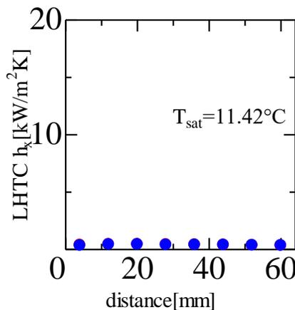
**Figure 11:** Local heat transfer coefficient of evaporation (mixture,  $x=0.99$ ,  $G = 10$  kg/m<sup>2</sup>s)
