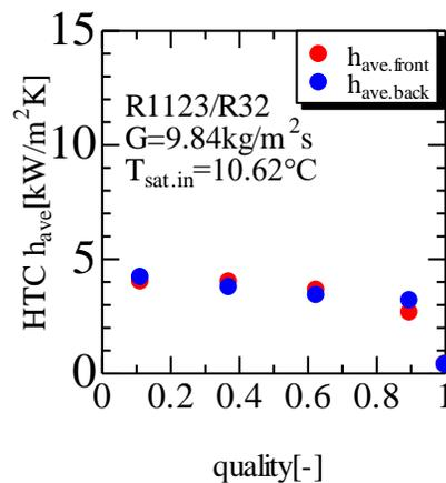
**Figure 12:** Average heat transfer coefficient of cross section (mixture,  $G = 10$  kg/m<sup>2</sup>s)
