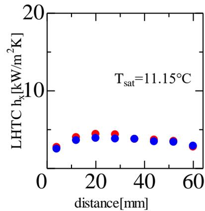
**Figure 10:** Local heat transfer coefficient of evaporation (mixture,  $x=0.62$ ,  $G = 10$  kg/m<sup>2</sup>s)
