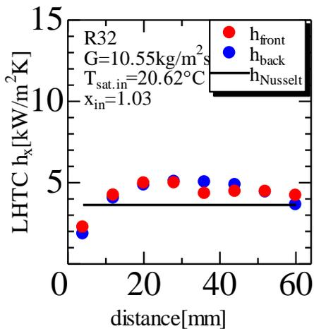
**Figure 7:** Local heat transfer coefficient of condensation (pure R32,  $x=0.92$ ,  $G = 10 \text{ kg/m}^2\text{s}$ )
