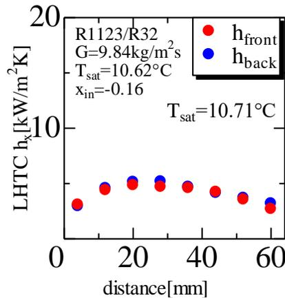
**Figure 9:** Local heat transfer coefficient of evaporation (mixture,  $x=0.11$ ,  $G = 10$  kg/m<sup>2</sup>s)
