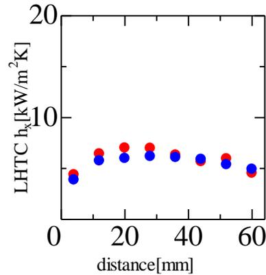
**Figure 14:** Local heat transfer coefficient of evaporation (pure R32,  $x=0.50$ ,  $G = 10 \text{ kg/m}^2\text{s}$ )
