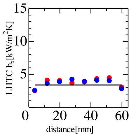
**Figure 8:** Local heat transfer coefficient of condensation (pure R32,  $x=0.57$ ,  $G = 10 \text{ kg/m}^2\text{s}$ )
