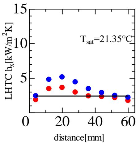
**Figure 5:** Local heat transfer coefficient of condensation (mixture,  $x=0.17$ ,  $G = 10 \text{ kg/m}^2\text{s}$ )
