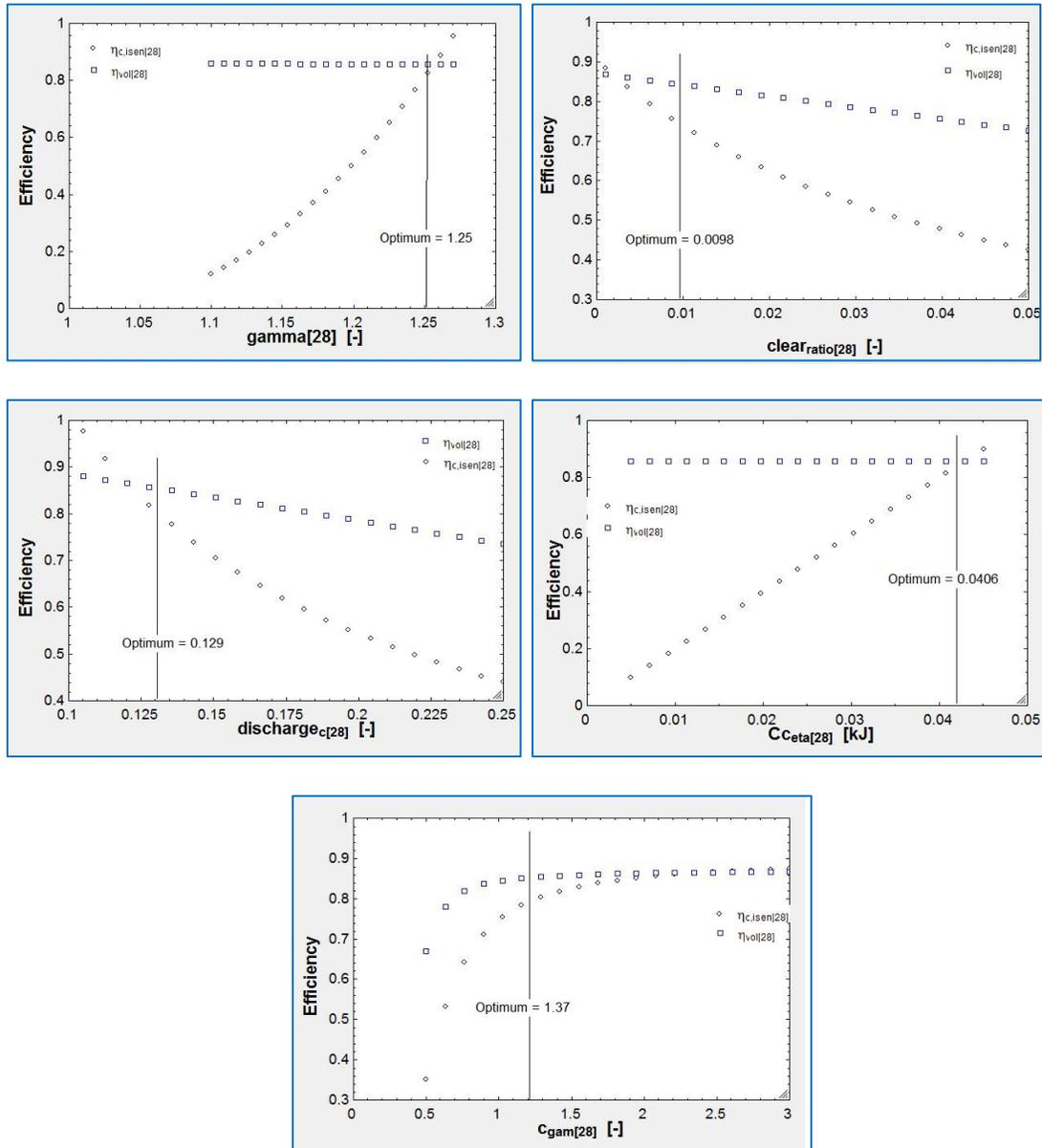
**Figure 1:** The variation of isentropic and volumetric efficiencies with the primary design variables of the system are as shown. The optimum values, based on minimum RMS error, for each design variable is identified on each plot.
