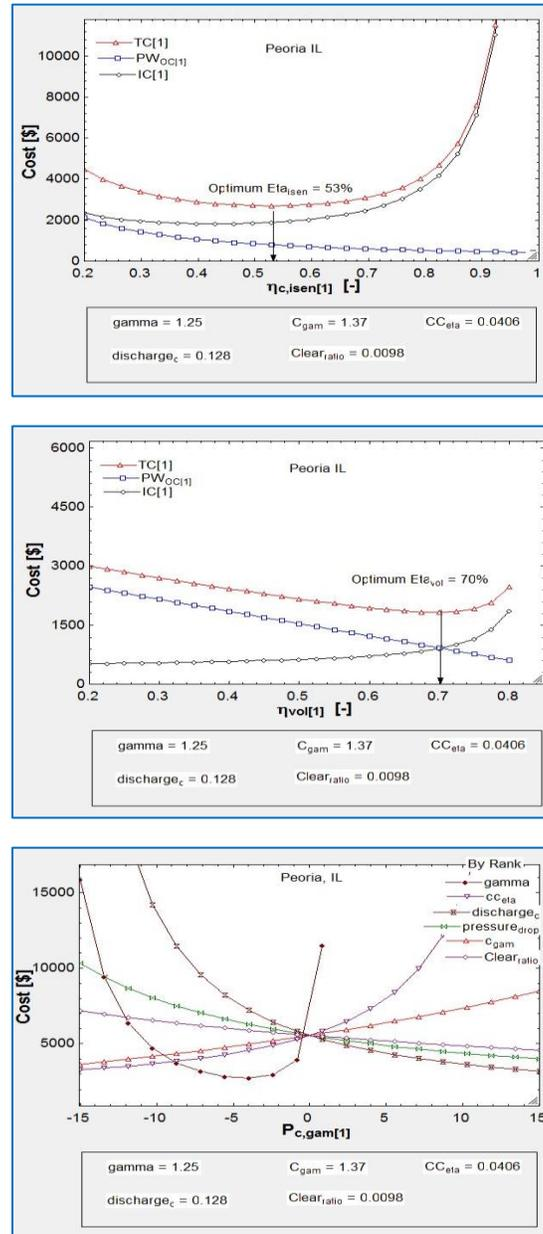
**Figure 5:** a) Graph shows the variation of initial (IC), operating (OC) and total life cycle cost (TC) with the isentropic efficiency of the compressor for Peoria, IL b) Graph shows the variation of initial (IC), operating (OC) and total life cycle costs (TC) with the volumetric efficiency of the compressor for Peoria, IL c) Graph shows the sensitivity of the Total costs to the primary design variables a compressor
