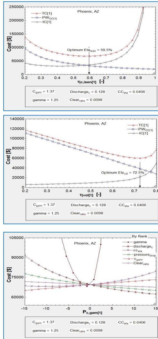
**Figure 4:** a) Graph shows the variation of initial (IC), operating (OC) and total life cycle cost (TC) with the isentropic efficiency of the compressor for Phoenix, AZ b) Graph shows the variation of initial (IC), operating (OC) and total life cycle costs (TC) with the volumetric efficiency of the compressor for Phoenix, AZ c) Graph shows the sensitivity of the Total costs to the primary design variables a compressor
