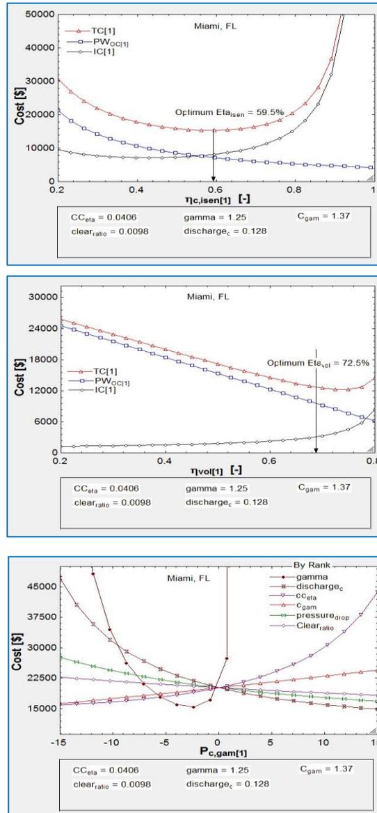
**Figure 7:** a) Graph shows the variation of initial (IC), operating (OC) and total life cycle cost (TC) with the isentropic efficiency of the compressor for Miami, FL b) Graph shows the variation of initial (IC), operating (OC) and total life cycle costs (TC) with the volumetric efficiency of the compressor for Miami, FL c) Graph shows the sensitivity of the Total costs to the primary design variables a compressor
