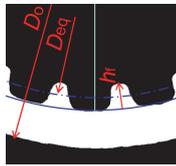
Figure 3: Cross-sectional view of test microfin tube
