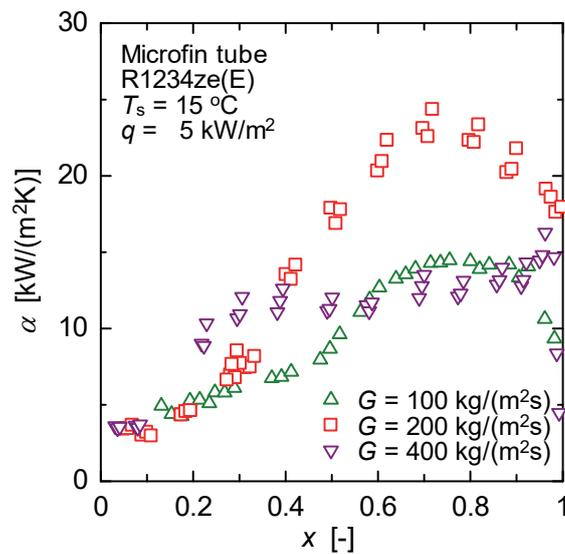
**Figure 5:** Effect of mass velocity on heat transfer coefficient at heat flux of 5 kW/m<sup>2</sup>
