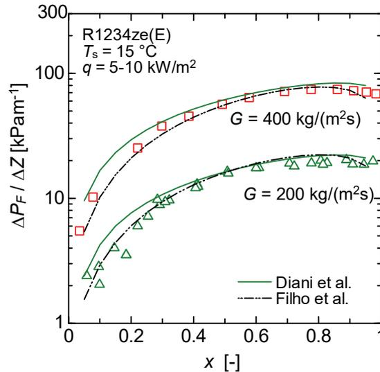
**Figure 8:** Frictional pressure drop at mass velocities of 200 and 400 kg/(m<sup>2</sup>s)
