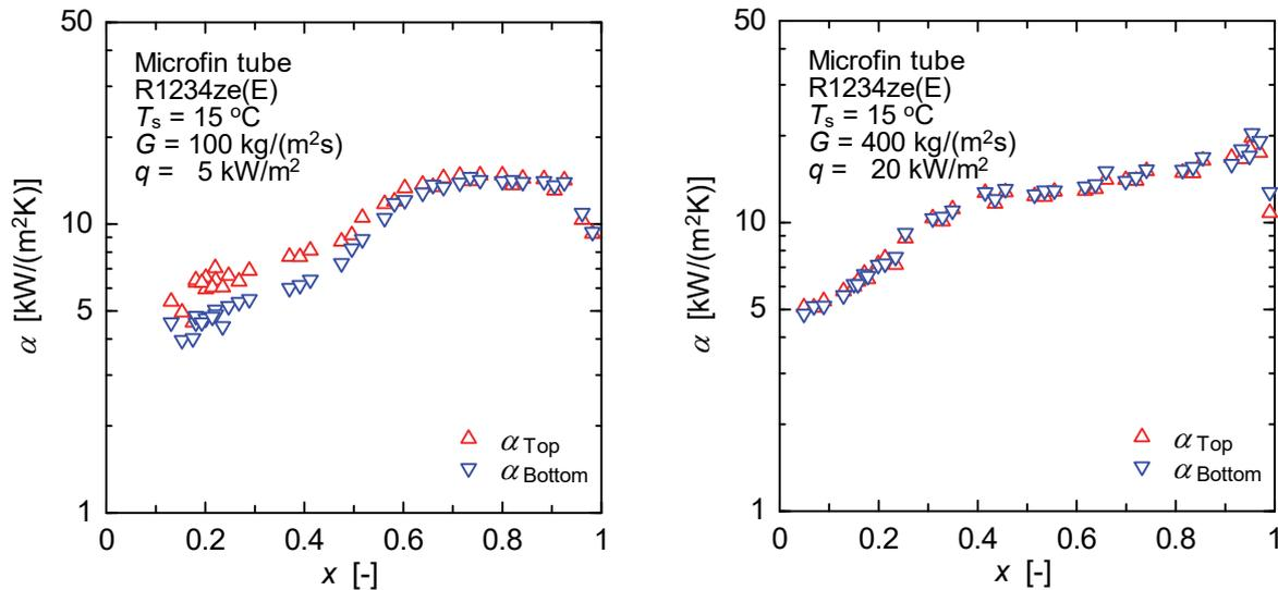
**Figure 6:** Difference of heat transfer coefficient between top and bottom sides of microfin tube at mass velocities of 100 and 400 kg/(m<sup>2</sup>s)
