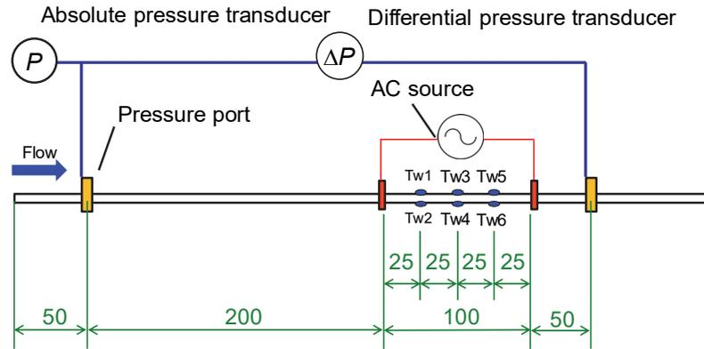
Figure 2: Details of test section
