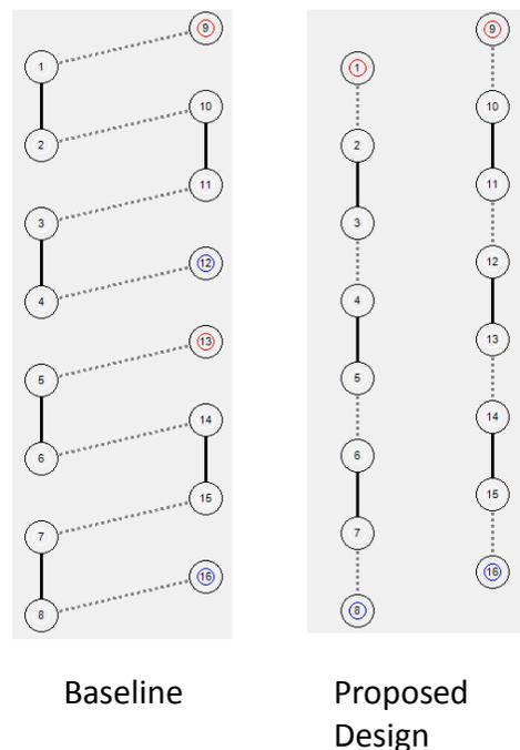
**Figure 3:** Condenser circuitry for baseline and proposed design
