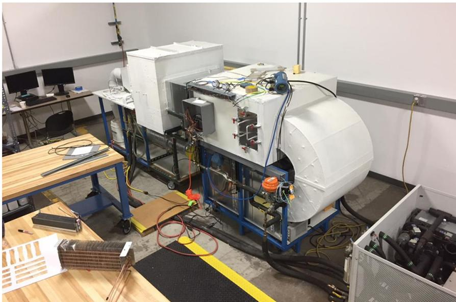
**Figure 6:** Hot water calorimeter
