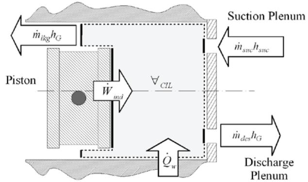
Figure 3. Control volume over the compression chamber.
