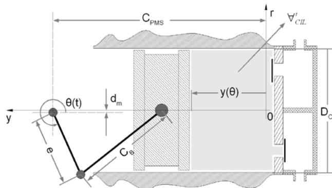
Figure 1. Schematic view of the compression chamber.
