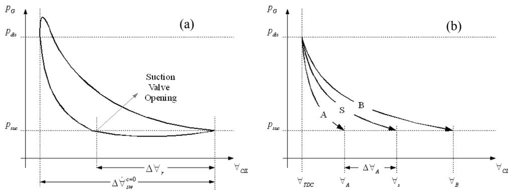
Figure 5. (a)  $p \times V$  Diagram showing the total swept volume and the volume swept during suction. (b) Three generic expansion processes.
