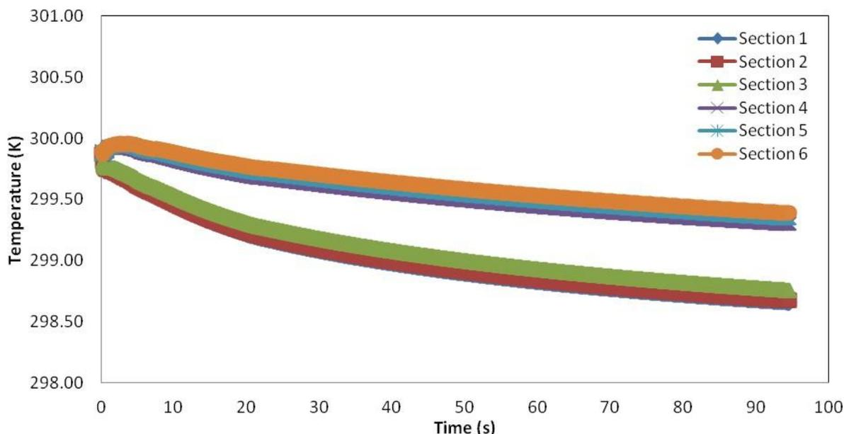
**Figure 6:** Average Insulation temperature for 0.5 inch insulation tank.
