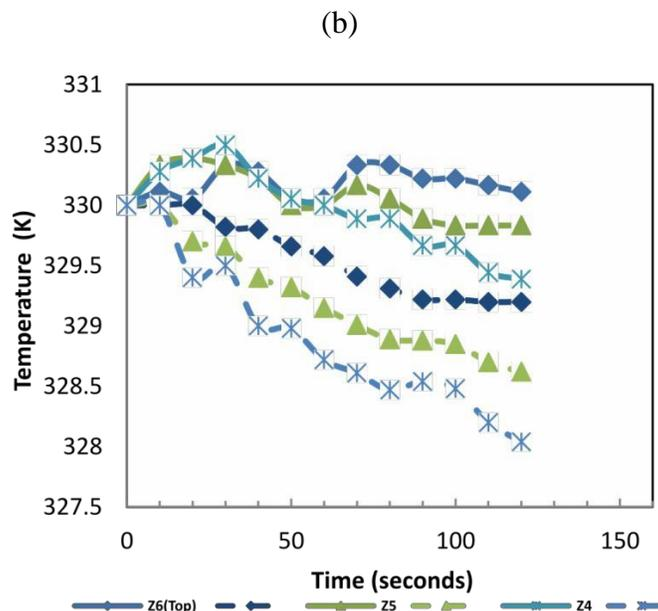
**Figure 3:** Comparison between measured values (solid lines) and numerical predictions (dotted lines) of water temperature along different heights (a)  $Z1=0$ ,  $Z2=0.19$  and  $Z3=0.36$ ) and (b)  $Z4=0.53$ ,  $Z5=0.7$  and  $Z6=0.89$  m)
