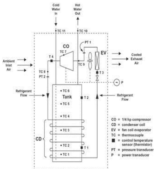
**Figure 1:** Schematic of heat pump system with wrapped coil tank.
