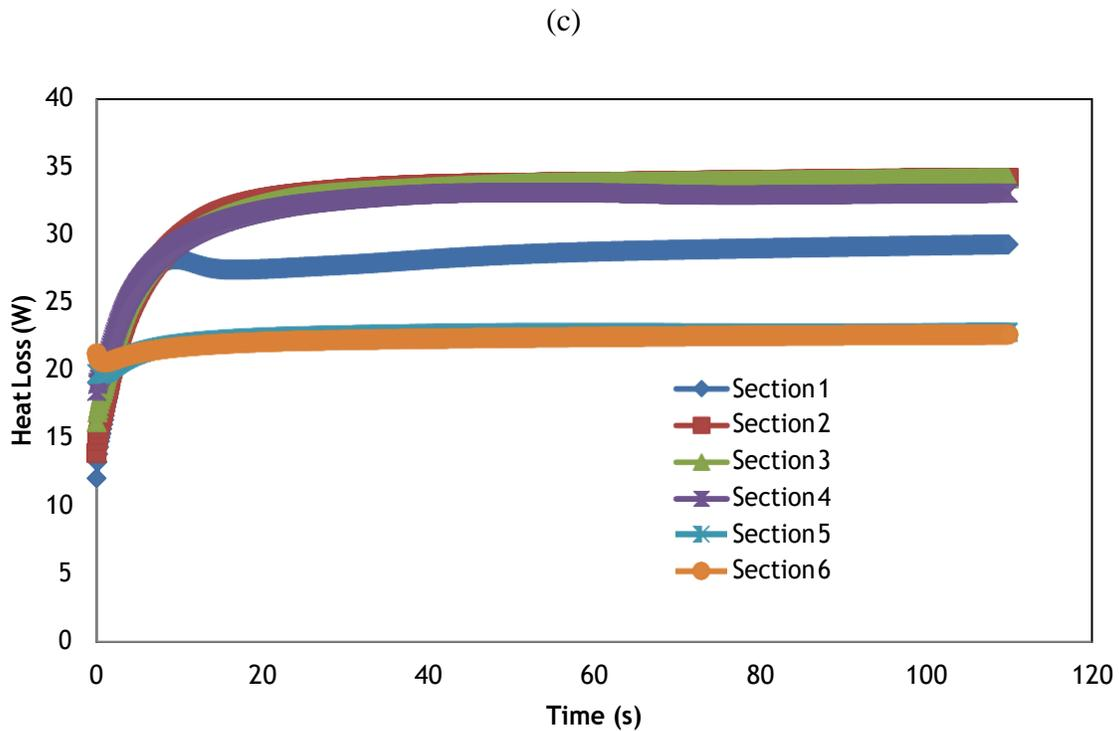
**Figure 4:** Average heat losses across the tank wall for (a) 0.5 inch insulation thickness, (b) 1 inch insulation thickness and (c) 2 inch insulation thickness.
