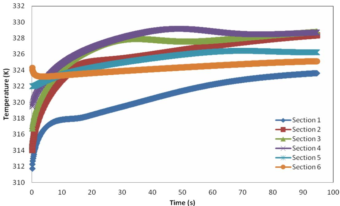
**Figure 5:** Average tank temperature with 0.5 inch insulation.
