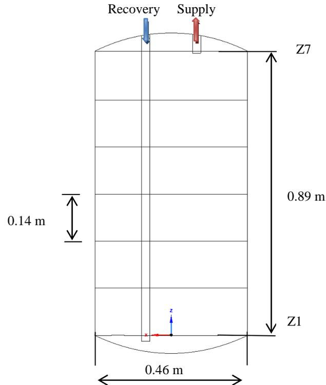
**Figure 2:** Water tank (Z1 to Z7 are the seven heights for temperature monitoring).
