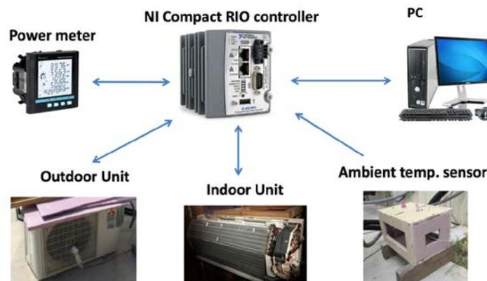
Figure 3: Experimental setup of the mini-split AC system
