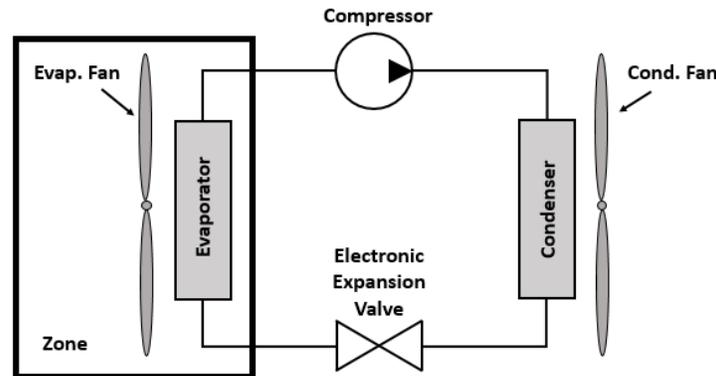
Figure 2: A simplified diagram of a mini-split AC system. There are four main components: 1) Compressor, 2) Electronic Expansion Valve (EEV), 3) Evaporator Fan, 4) Condenser Fan
