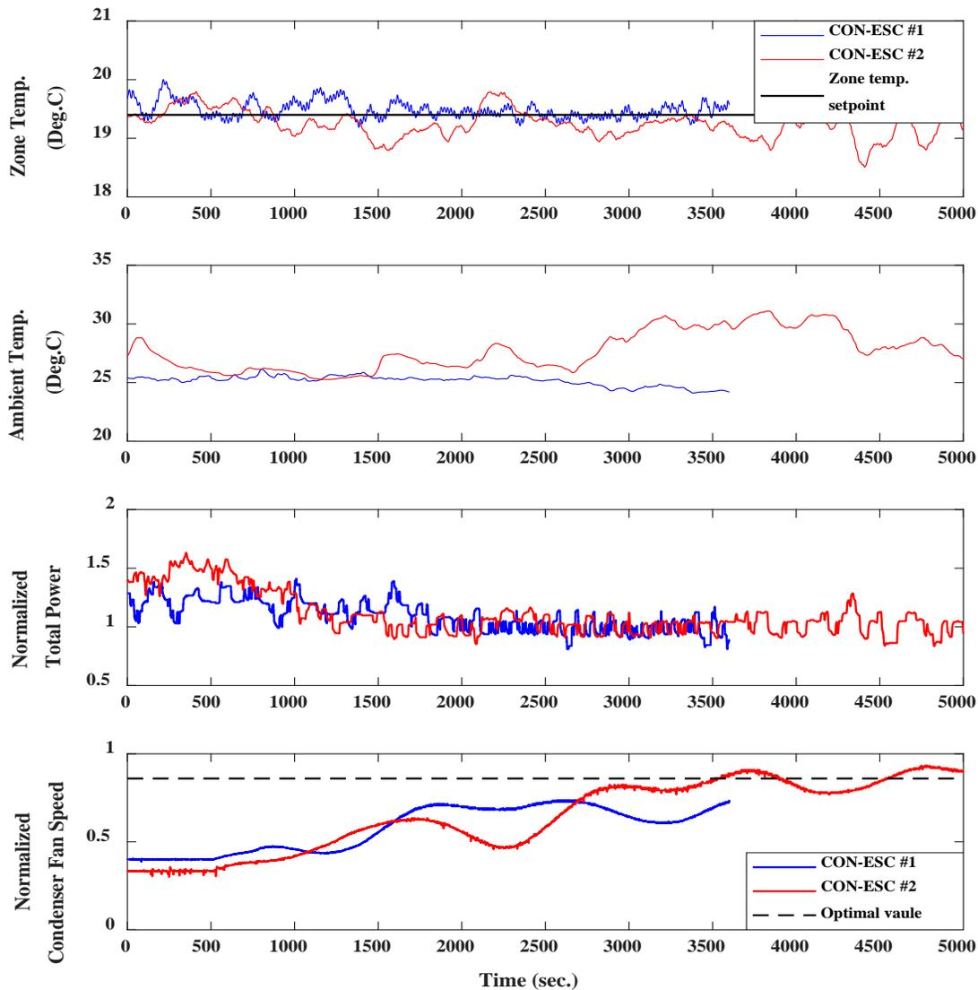
**Figure 6.** Testing results of single-input CON-ESC: normalized input/output trajectories, zone and ambient temperatures.
