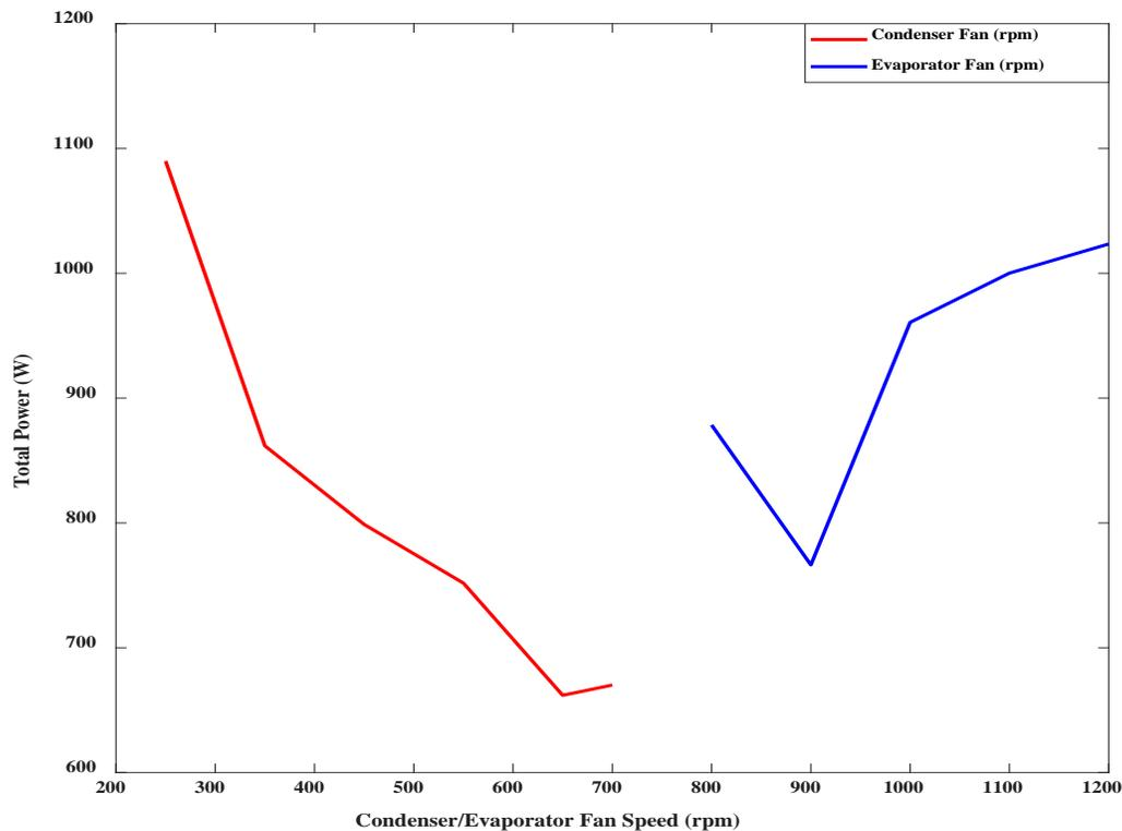
Figure 4: Static map of total power as a function of condenser and evaporator fan speed
