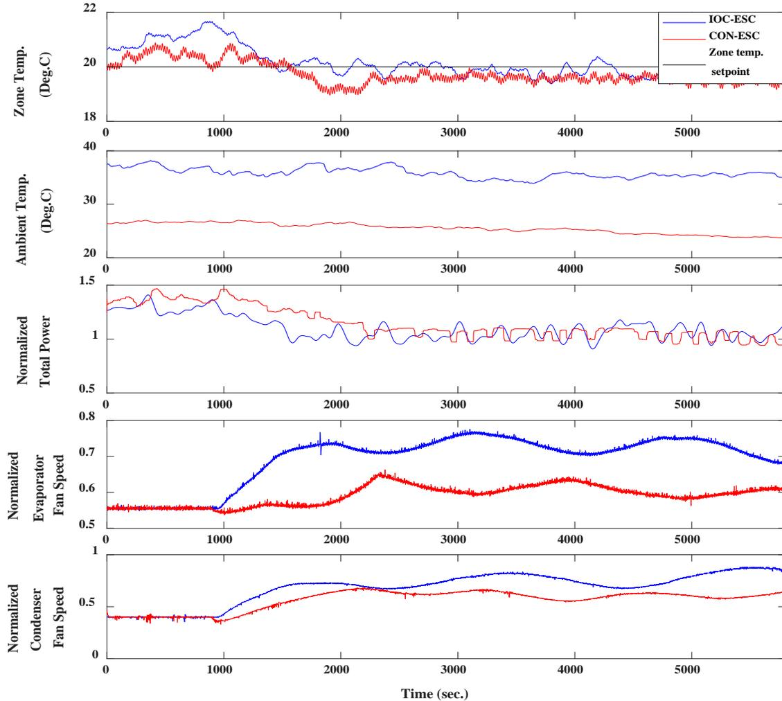
**Figure 7.** . Testing results of two-input IOC-ESC I/O trajectories and two-input CON-ESC
