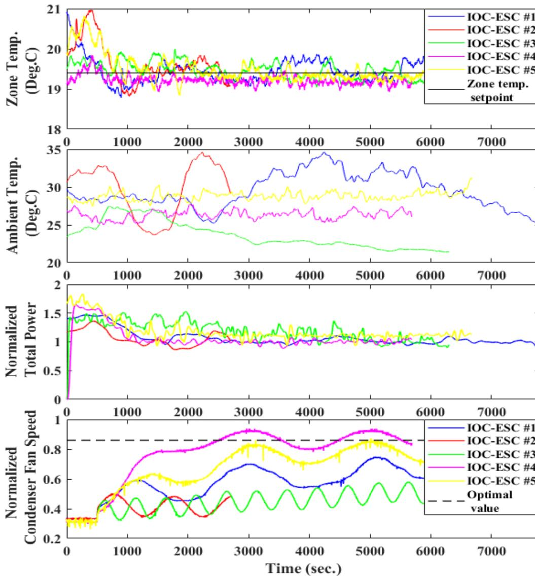
**Figure 5.** Testing results for single-input IOC-ESC: normalized input/output trajectories, zone and ambient temperatures.
