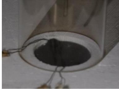
**Figure 5-** Image showing chimney above planchette at a specified gap height
