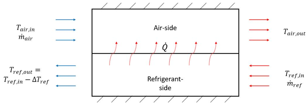
**Figure 2:** Segmented Counter-Flow Heat Exchanger Modeling Diagram
