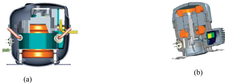
Figure 2: HFC compressor (a) present expressive differences when compared to CO 2 compressor.
