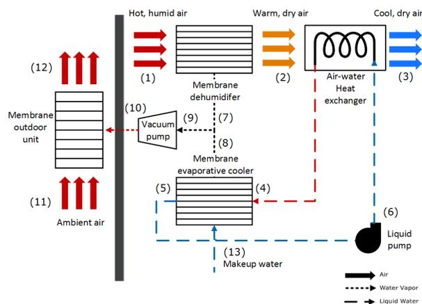
Figure 1: Schematic of membrane heat pump system
