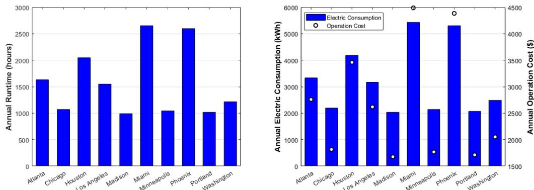
**Figure 5:** (a) Membrane system annual runtime, (b) Membrane system annual electric consumption and operation costs
