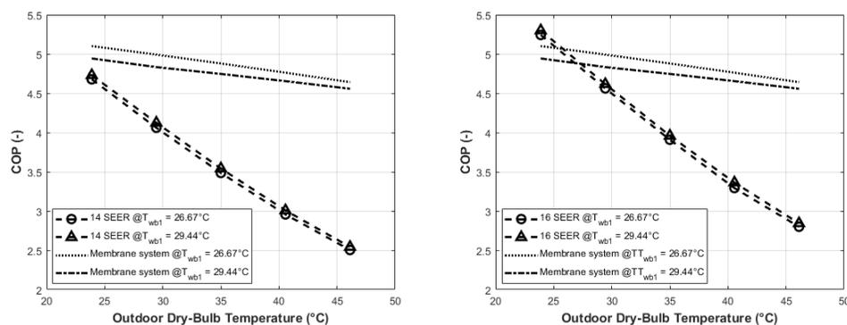
**Figure 6:** (a) Comparison between the membrane system and 14 SEER vapor compression system, (b) Comparison between the membrane system and 16 SEER vapor compression system
