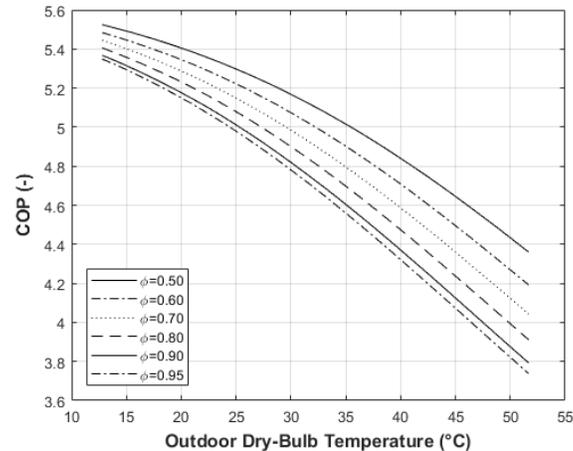
**Figure 2:** Membrane system COP versus dry-bulb temperature at different relative humidity
