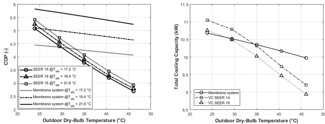
**Figure 7:** (a) Indoor unit's wet-bulb temperature effect on system's COP (b) Total cooling load provided by the 3 systems at different outdoor dry-bulb temperature
