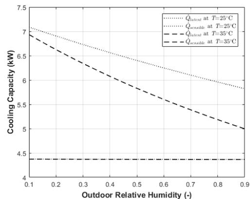
**Figure 3:** Membrane system cooling loads evaluated at different outdoor conditions
