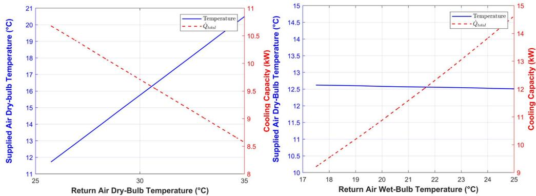
**Figure 4:** (a) Supplied air dry-bulb temperature at varied return air dry-bulb temperatures, (b) Supplied air dry-bulb temperature at varied return air wet-bulb temperatures
