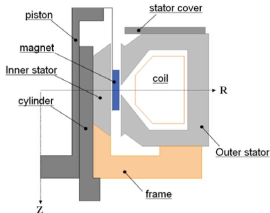
Figure 4: Analysis model of linear motor system
