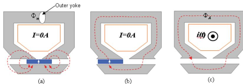
Figure 2: Magnetic flux path of linear motor
