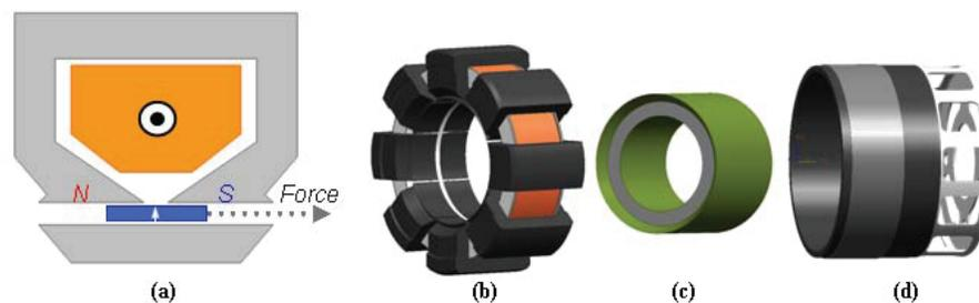
Figure 1: Linear oscillating motor
