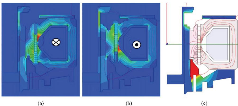
Figure 6: Distributions of coil current field and eddy current loss
