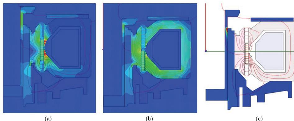
Figure 5: Distributions of magnet field and eddy current loss
