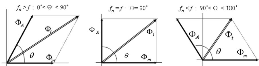
Figure 3: Phase diagrams of magnet and coil flux
