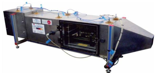
Fig.1b: Sensor layout profile on Edibon tray drier [16].
