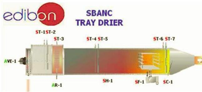
Fig.12: Layout of sensors in drier unit.
