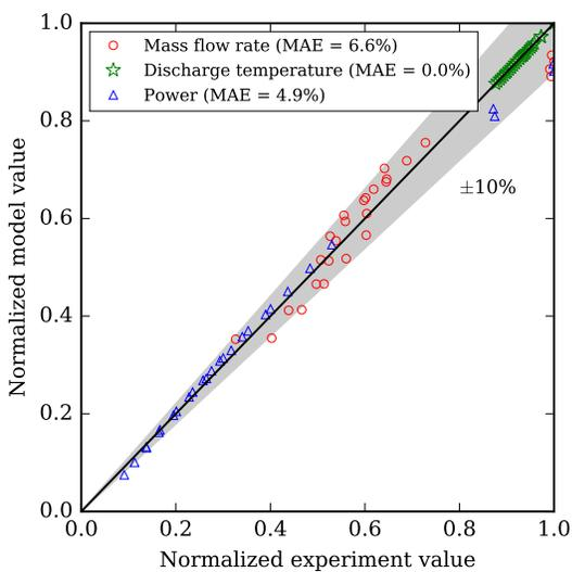
Figure 3: Validation of variable-speed rolling piston compressor.
