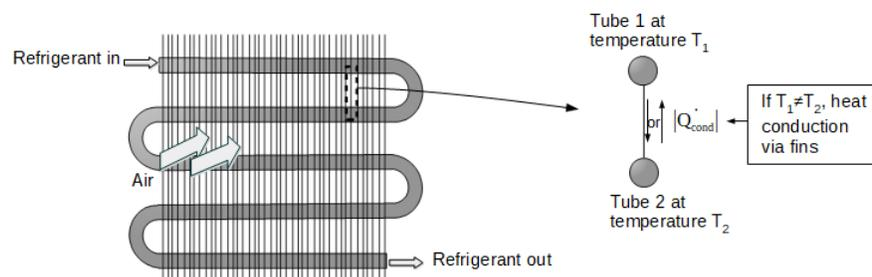
Figure 3: Tube to tube (or cross fin) conduction
