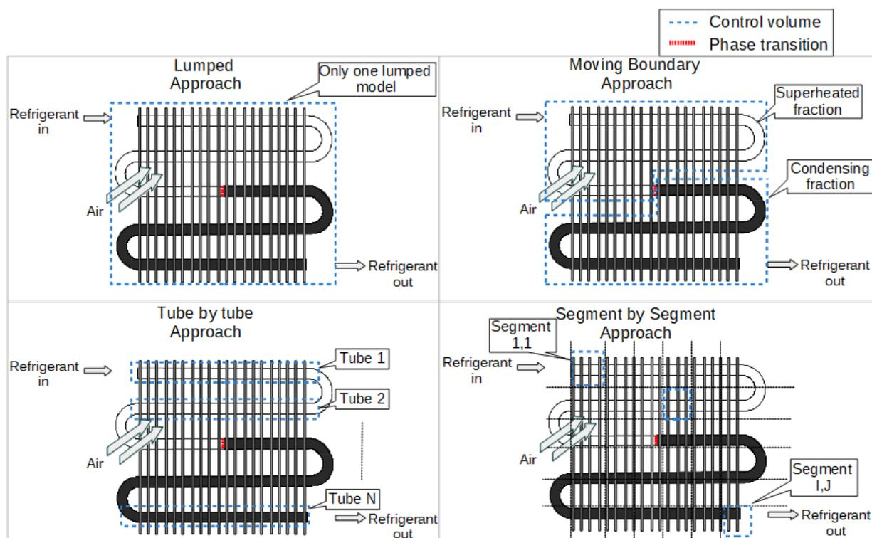
Figure 2: Control volume for different modeling approaches
