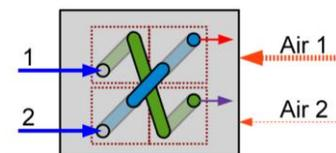
Figure 4: Refrigerant circuitry interleaved (Bach *et al.* 2014b)
