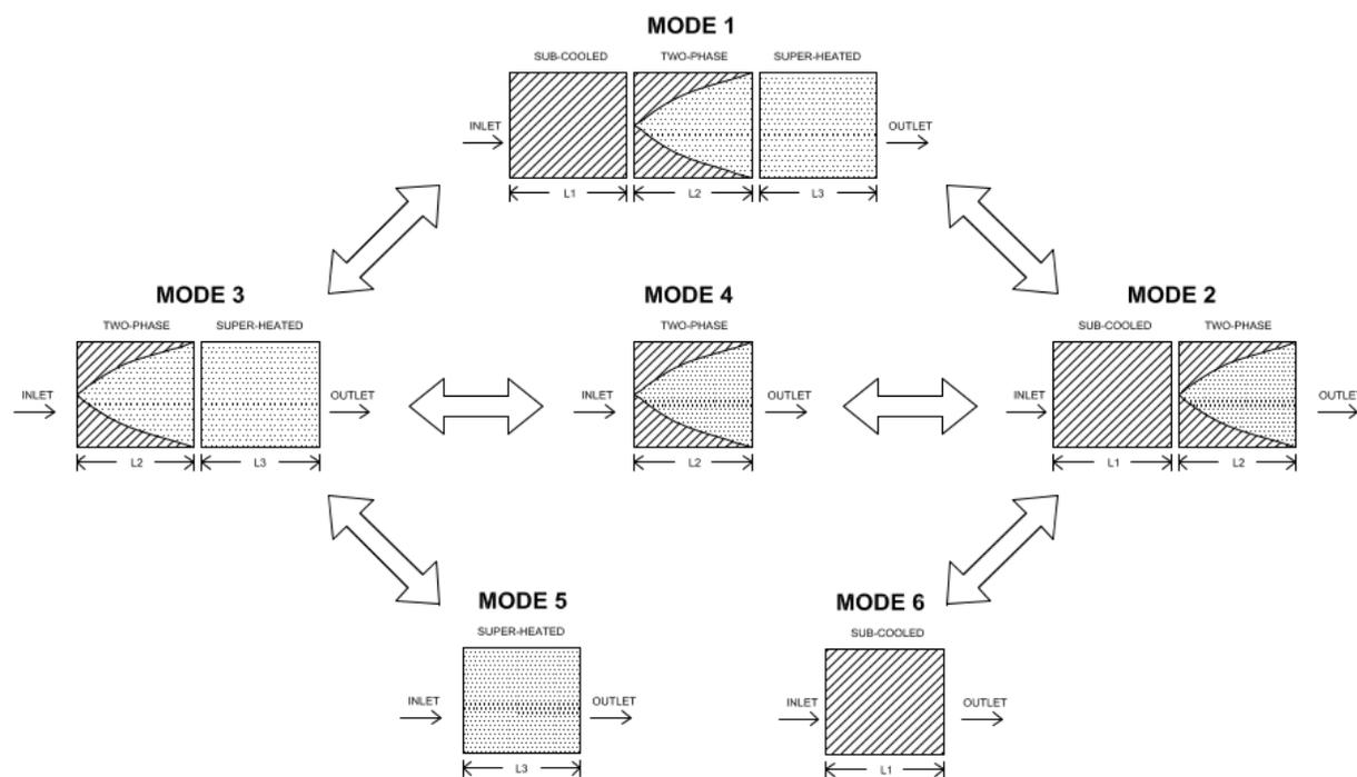
**Figure 2:** SMB approach: evaporator modes and transitions
