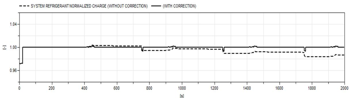
**Figure 9:** Refrigerant charge conservation. System cyclic on/off simulation
