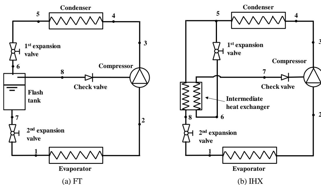
Fig. 1 Schematic diagram gas injection systems
