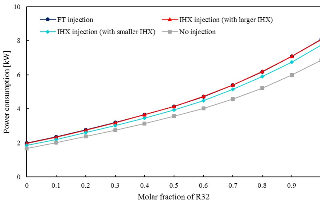
**Figure 4:** Power consumption of FT system, IHX system and no injection systems
