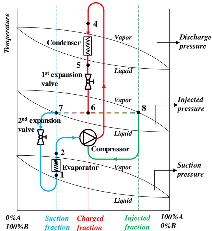
Fig. 2 Temperature-fraction diagram of FT gas injection system with zeotropic refrigerant
