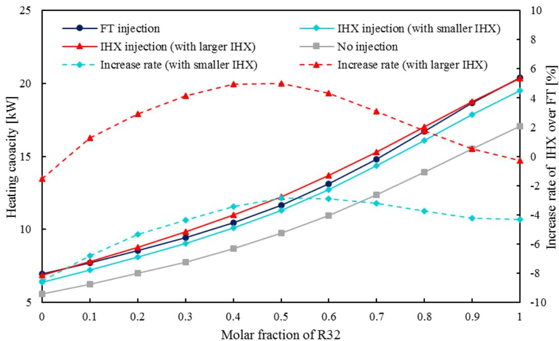
**Figure 3:** Heating capacity of FT system, IHX system and no injection systems
