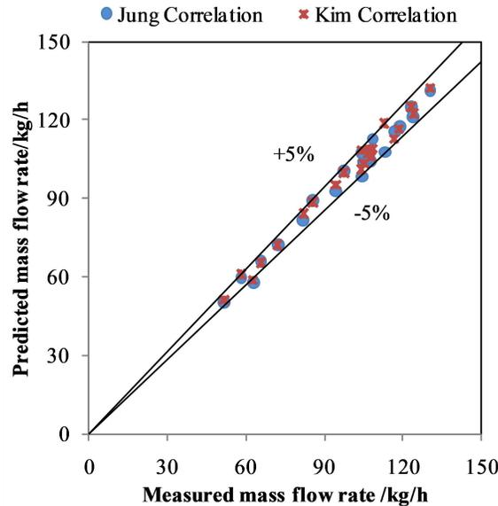
Figure 2: Comparison of measured data and predicted data for capillary tubes
