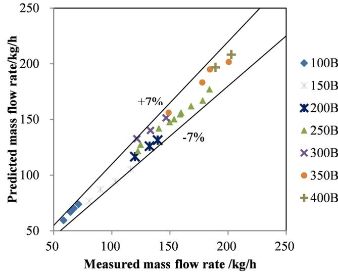
Figure 3: Comparison of measured data and predicted data for EEV
